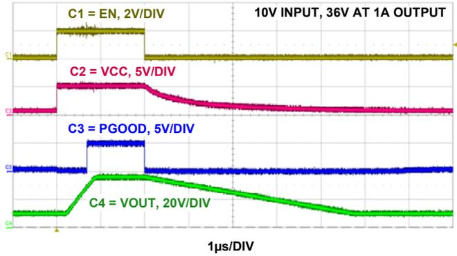
FIGURE 11. ENABLE/DISABLE WAVEFORMS
