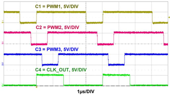
FIGURE 9. WAVEFORMS WITH PWM\_INV = V<sub>CC</sub>
