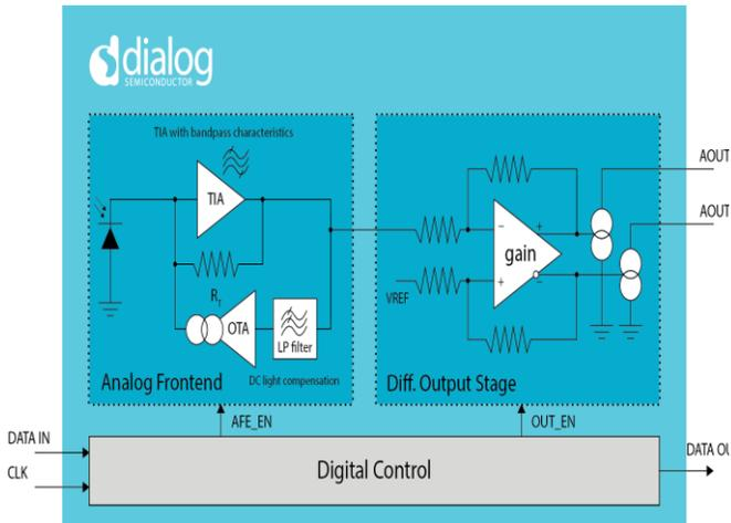
To select the correct photodiode for this application, Renesas proposed several solutions to our customer. These photodiodes were designed, manufactured and tested by Renesas and the version that best fit the requirements was selected for use in the custom chip. The next stage in the process was integrating these photodiodes with the rest of the required circuitry for the final ASIC. The additional circuitry included a dedicated AFE and transimpedance amplifier.
