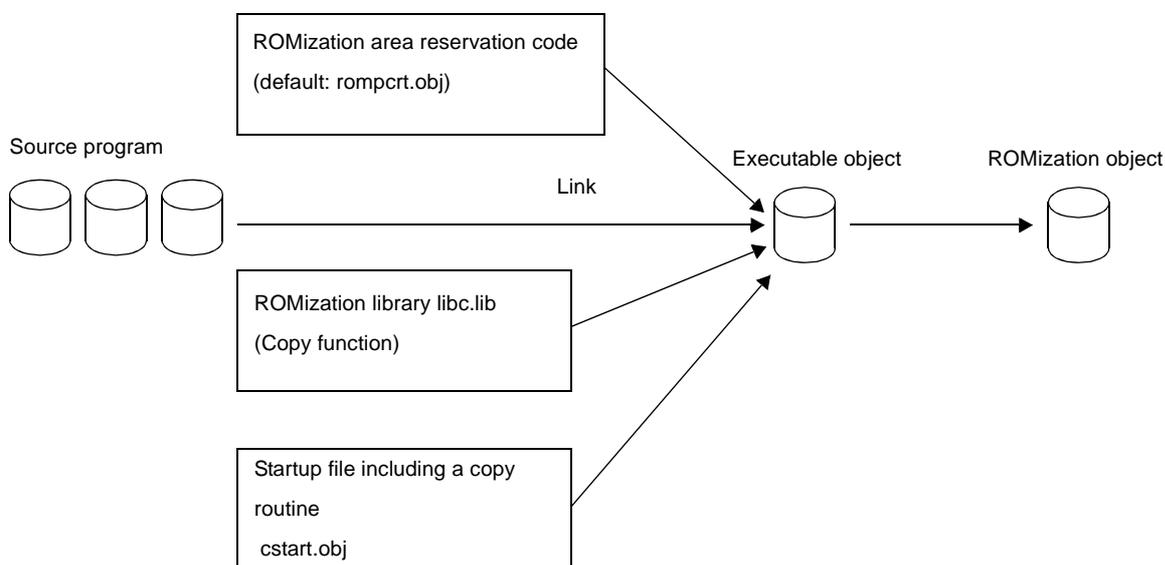
When ROMization objects are created as shown in the "Figure 8-1. Creation of Object for ROMization", execution of the `_rcopy` copies the data to be allocated to RAM from the packed ROM section.
