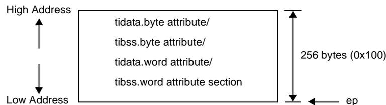
Data with initial values is allocated to the tidata (tidata.byte, tidata.word) attribute section, and data without initial values is allocated to the tibss (tibss.byte, tibss.word) attribute section. Specify the tidata.byte/tibss.byte attribute to allocate byte data, and specify the tidata.word/tibss.word attribute to allocate word data. To select automatic byte/word judgment by the CX, specify the tidata/tibss attribute.
