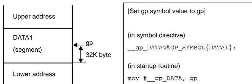
In the above example, the link directive is used to set so that the gp symbol value references the DATA1 segment. Since the gp symbol name is "\_\_gp\_DATA", the address that is 32K-byte away from the start of the DATA1 segment which is determined when linking is set to the symbol "\_\_gp\_DATA" (see "Figure 5-6. Example of gp Setting (When Specifying Segment)").
