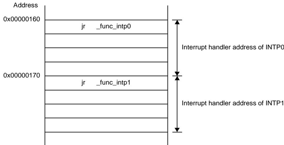
If the INTP0 interrupt occurs in the V850E2/MN4, the program jumps to address 0x160 and executes the code written at that address. In this example, the program jumps to the func\_intp0 function because a code that branches to that function is written. This means that func\_intp0 is the interrupt handler of INTP0.
