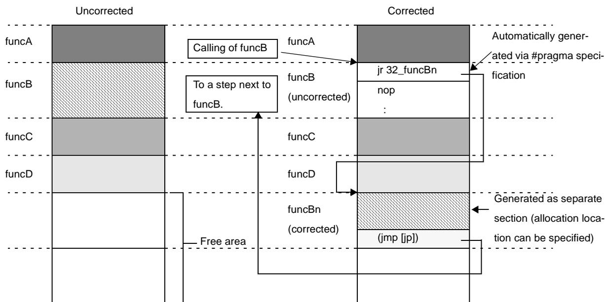
The smart correction feature is useful when a bug is found in a specific function after the program has been written to the flash area.
