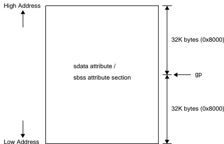
In many cases, however, variables exceed in this range when using an application that uses many variables. In this case, the variables must be allocated to other sections. The CX has many sections to which variables and data can be allocated, in addition to the sdata and sbss attribute sections. Each of these sections has its own feature and sections to which variables that must be accessed quickly can be allocated are also available, so that the sections can be selected depending on the usage.
