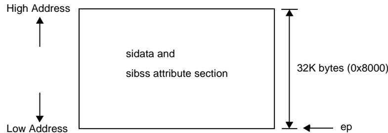
Data with initial values is allocated to the `sidata` attribute section, and data without initial values is allocated to `sibss` attribute section. If variables that exceed the upper limit of the `sdata` and `sbss` attribute sections that can be accessed from `gp` with 1 instruction, but which need to be accessed with 1 instruction still exist, they can be allocated in the range that can be accessed with 1 instruction using `ep`.
