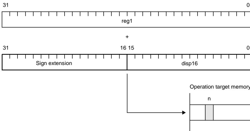
**Remark** n: Bit position specified with 3-bit data (bit#3) (n = 0 to 7)
