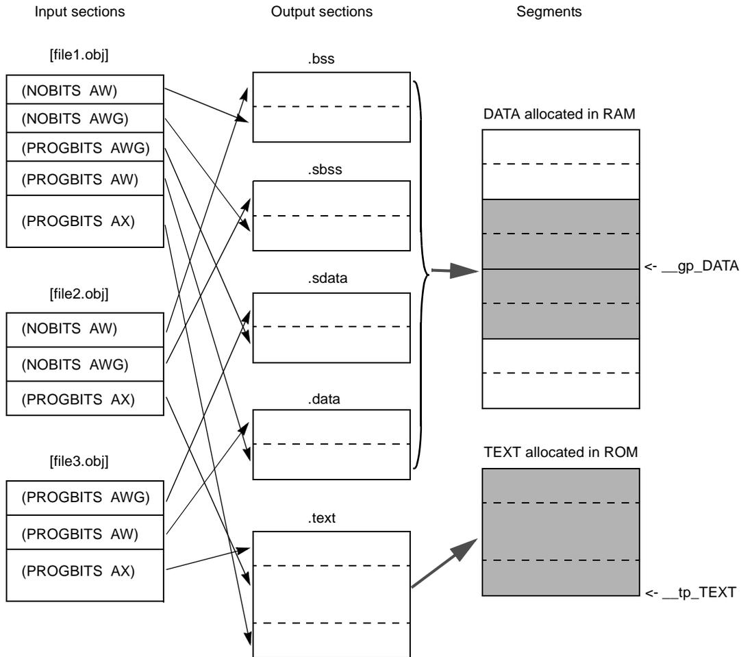
Sections that are included in objects (file1.obj, file2.obj, file3.obj) are called "input sections". These sections are gathered in the same attribute. Sections that are grouped and output are called "output sections". Output section groups are also gathered in corresponding segments (DATA segment and TEXT segment) and are mapped to appropriate areas (if there is no explicit address specification).
