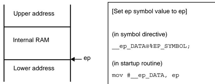
In the above example, the link directive is used to declare the creation of an ep symbol. Since the ep symbol name is "\_\_ep\_DATA", the linker sets the start address of internal RAM to "\_\_ep\_DATA".
