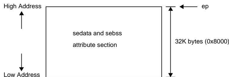
Data with initial values is allocated to the sedata attribute section, and data without initial values is allocated to the sebss attribute section. If variables that exceed the upper limit of the sdata and sbss attribute sections that can be accessed from gp with 1 instruction, but which need to be accessed with 1 instruction still exist, they can be allocated in the range that can be accessed with 1 instruction using ep.
