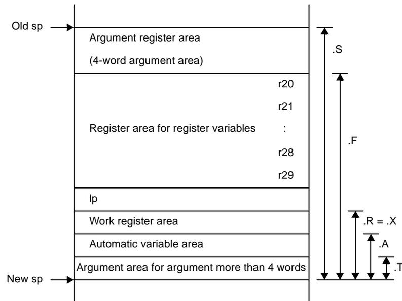
".S, .F, .X, .R, .A, and .T" in the figure are macros for functions output by the compiler internally. macros are used for a specific purpose, as shown in the following table.
