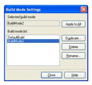
Select the build mode to be changed from the build mode list. The selected build mode will be displayed in [Selected build mode].
