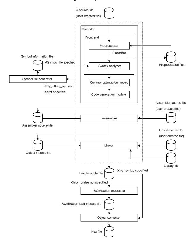
Figure B-1. Operation Flow of cx
