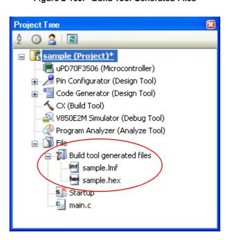
Figure 2-109. Build Tool Generated Files
