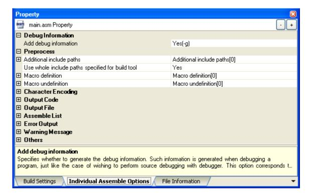
You can set assemble options for the assembler source file by setting the necessary properties in this tab.
