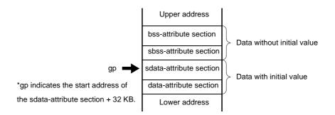
Therefore, the execution efficiency and object efficiency are enhanced if more data is allocated to the sdataattribute or sbss-attribute section, which can be accessed with a single instruction.
