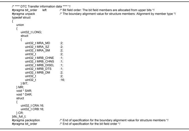
Figure 6.4 Structure/Union Used in the Sample Code
