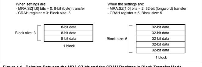
Figure 4.1 Relation Between the MRA.SZ bit and the CRAH Register in Block Transfer Mode
