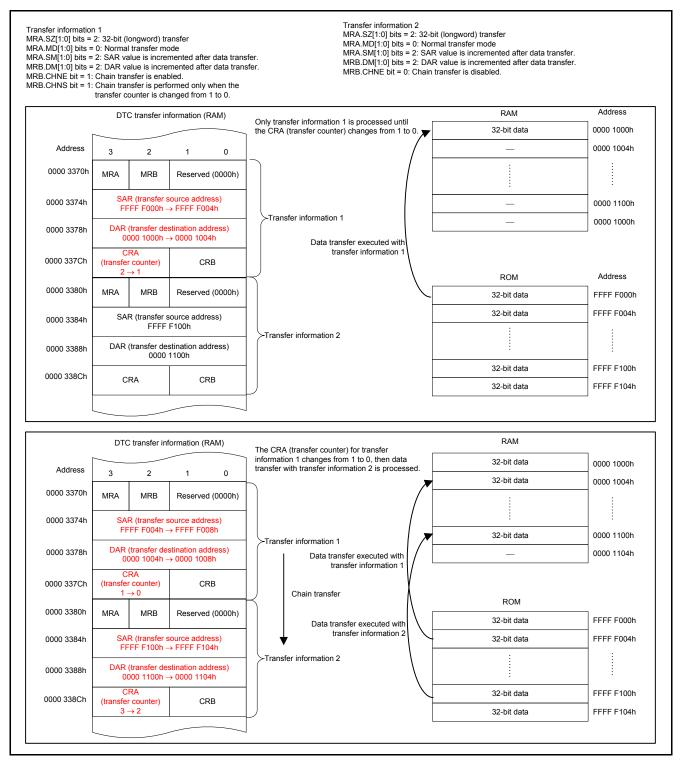
Figure 4.3 Chain Transfer in Normal Transfer Mode
