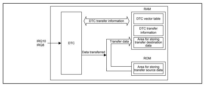
Figure 1.1 Block Diagram
