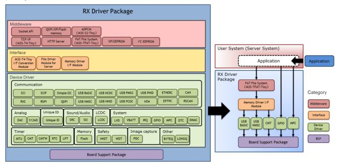
Figure 1-1 An Example of System Build
