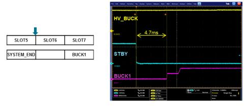
Figure 6: STBY Sequencing Control in Power-Down Mode
