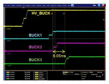
Figure 3: Sequencing Waveform
