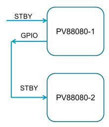
Figure 8: Multiple PV88080 Connection
