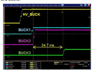
Figure 5: Sequencing with Additional WAIT\_STEP Slot
