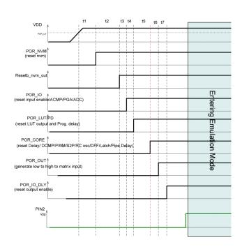
Figure 5. GreenPAK2 Startup
