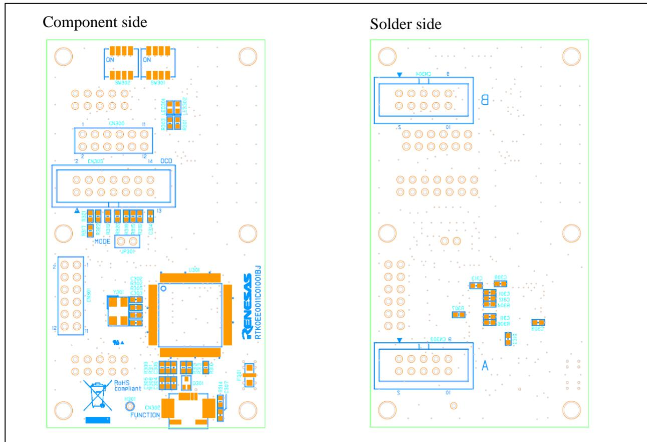
Figure 3-4 RX651 MCU board parts layout and silkscreen
