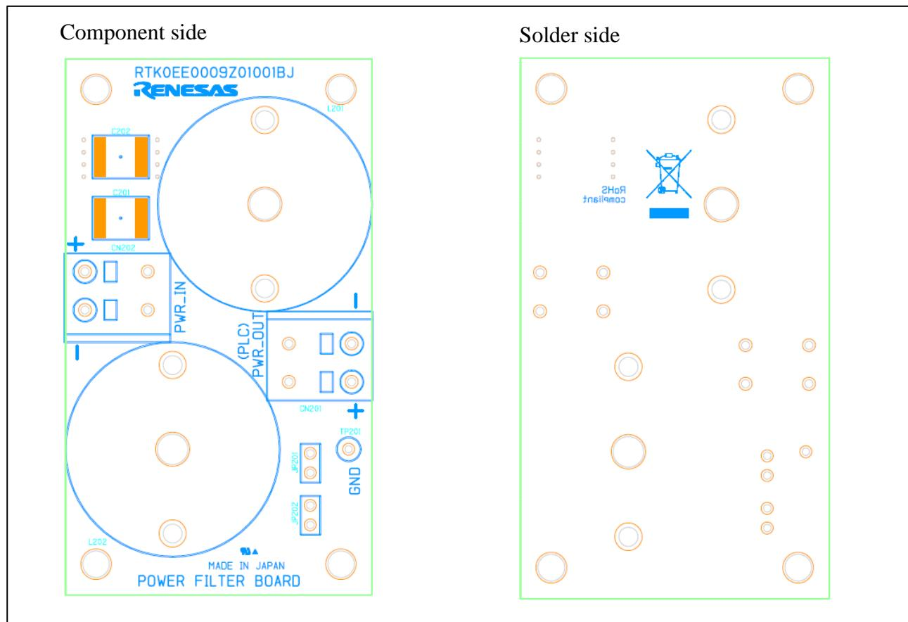
Figure 3-6 Power Filter board parts layout and silkscreen
