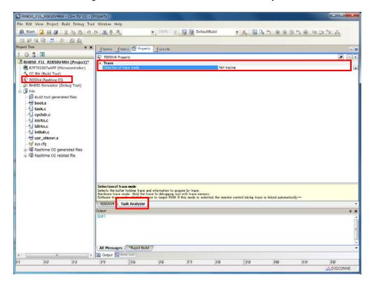
figure 9-10 Select Trace Mode on the Task Analyzer
