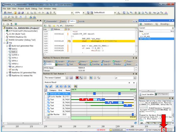
figure 9-13 Enable The Trace Function of The Debugger
