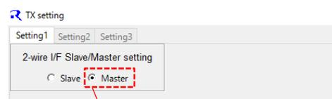
Figure 3.3 2-wire serial communication interface Slave/Master setting of TxIC in control tool
