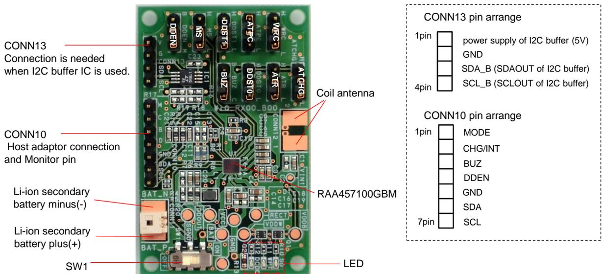
Figure 5.3 Name and function of receiver board
