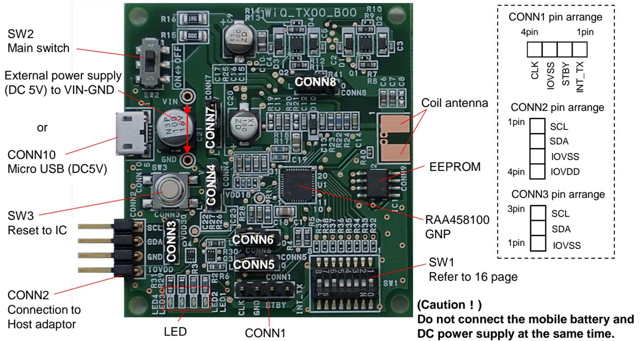
Figure 5.1 Name and function of transmitter board
