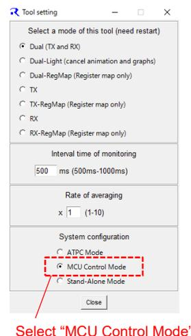
Figure 4.2 Tool window after start up
