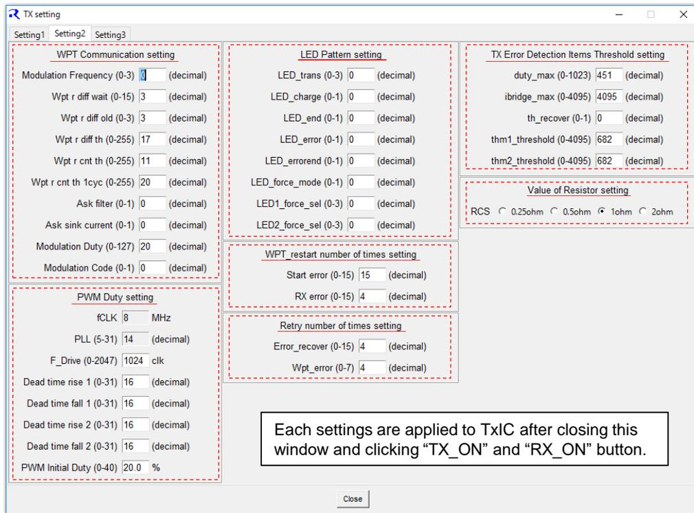
Figure 6.4 TX setting\_Setting2
