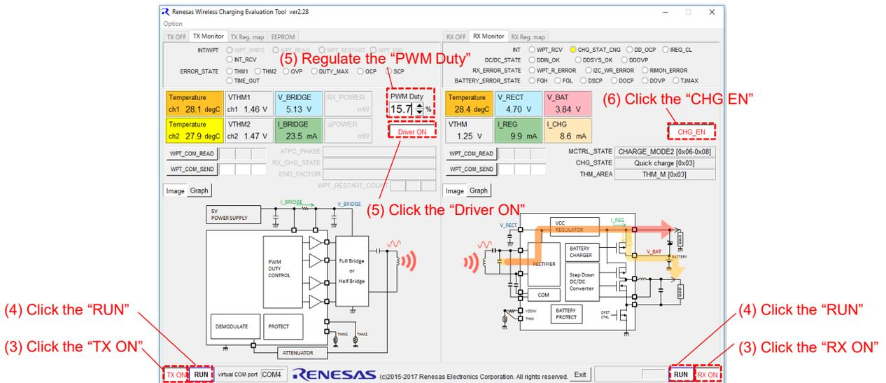
**Figure 4.3 Control tool window in MCU Control Mode**
