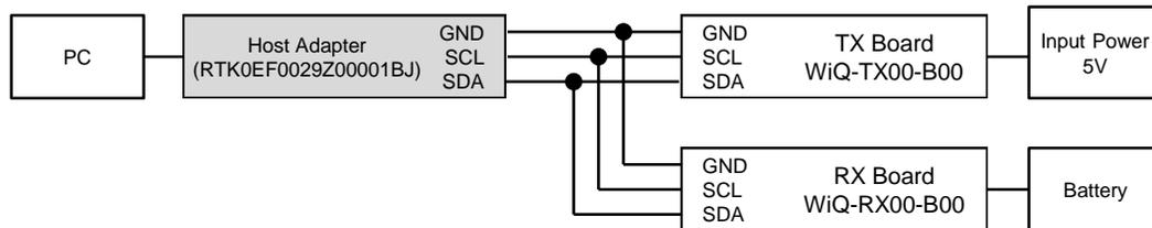
Figure 1.3 Connection of the host adaptor
