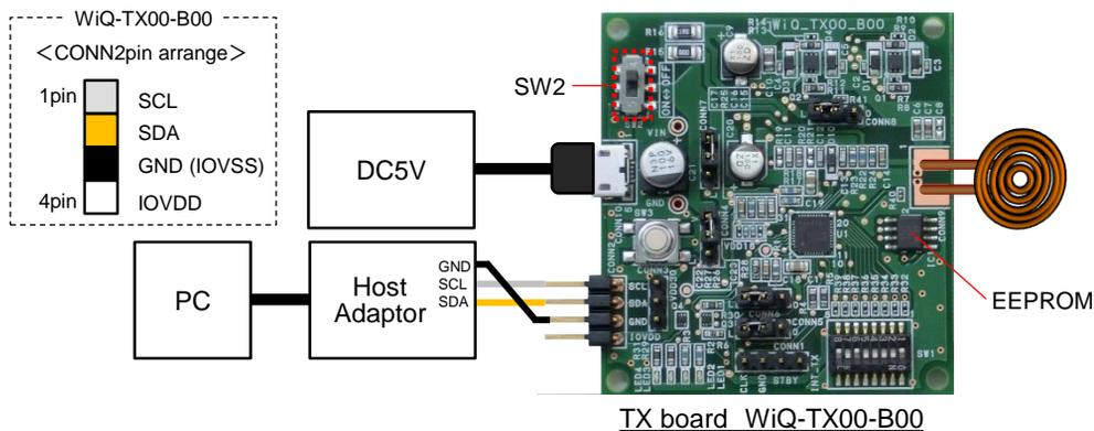
Figure 3.2 Connection in writing and reading EEPROM
