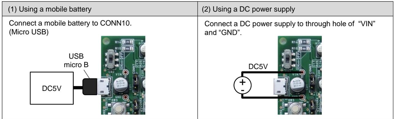
Figure 1.2 Connection method of power supply to WiQ-TX00-B00
