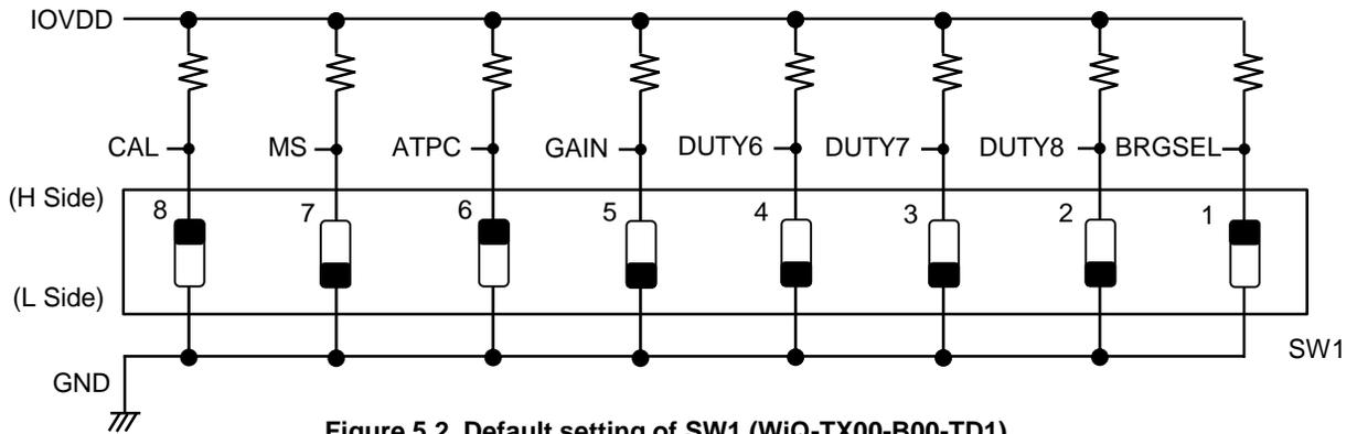
Figure 5.2 Default setting of SW1 (WiQ-TX00-B00-TD1)
