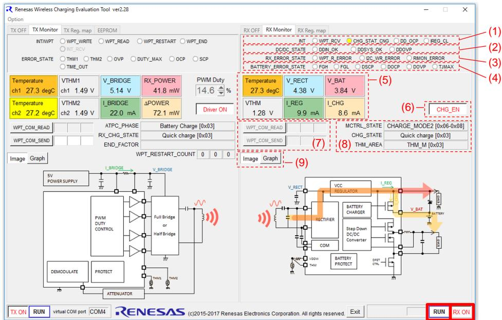
Figure 6.9 RX side window on main view
