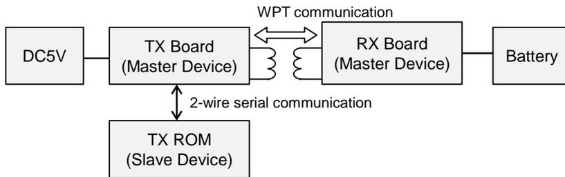
Figure 3.1 Evaluation system in AT1
