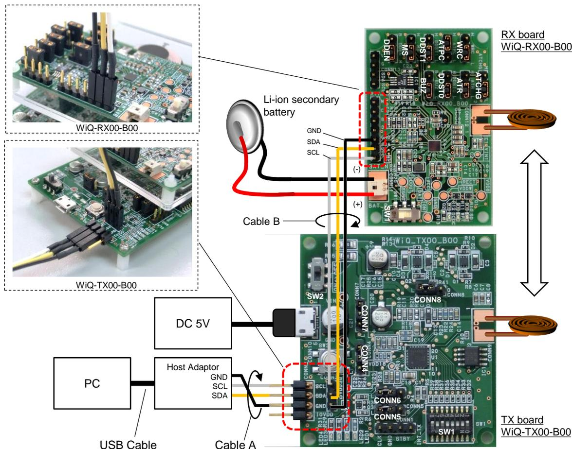
Figure 1.1 Connection of Wireless charging evaluation kit
