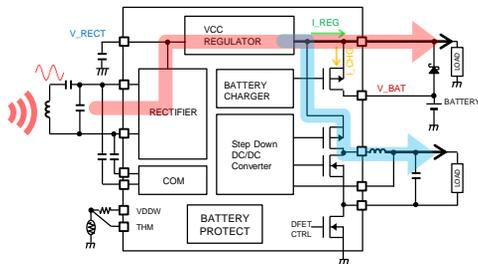
Battery is charged and DCDC converter is operating.
