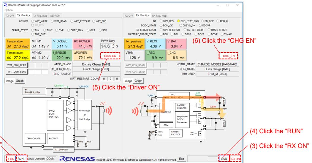
**Figure 2.3 Control tool window at ATPC Mode**
