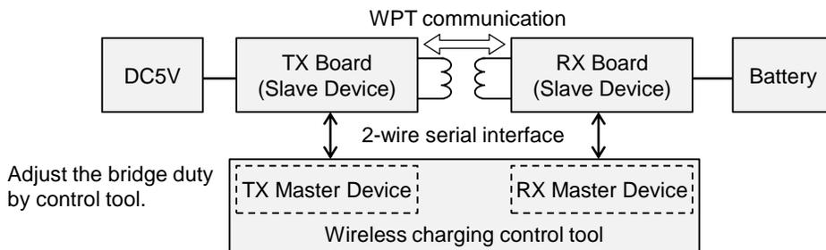
Figure 4.1 Evaluation system in MC1
