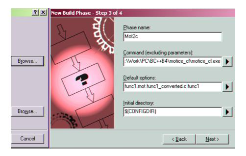
Here the phase has been called 'Mot2c', the full path for the 'Motice\_cl' executable has been entered as have the default parameters for the command. In this case the default parameters are the command line parameters for the utility.
