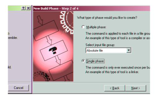
5. Configure the build phase to call 'Motice\_cl' with the correct command line parameters.
