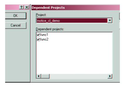
Now, whenever the 'motice\_cl\_demo' project is built both the 'func1' and 'func2' projects will be built first and so ensuring that very latest converted files are made available to 'motice\_cl\_demo.
