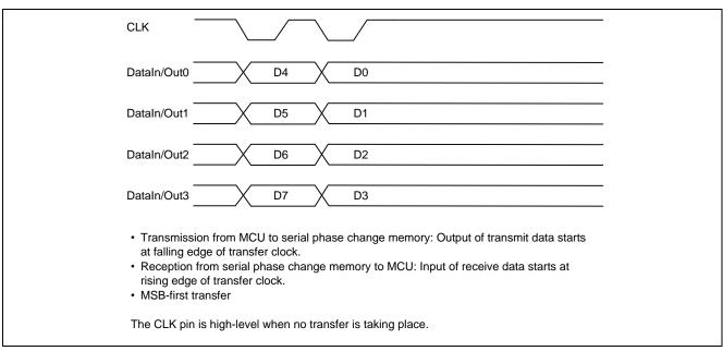
Figure 5.4 Quad-SPI Clock Synchronous Mode Timing Settings
