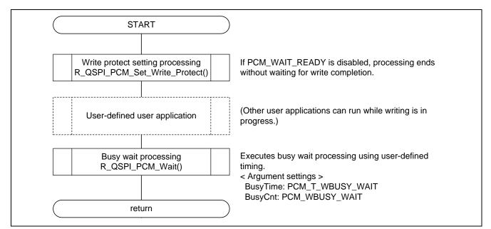
Figure 5.11 Using R\_QSPI\_PCM\_Wait() to Wait for Write Protect Setting Completion
