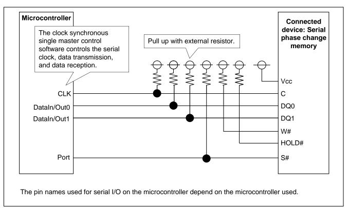
Figure 4.2 MCU and SPI Slave Device Connection Example for Dual-SPI
