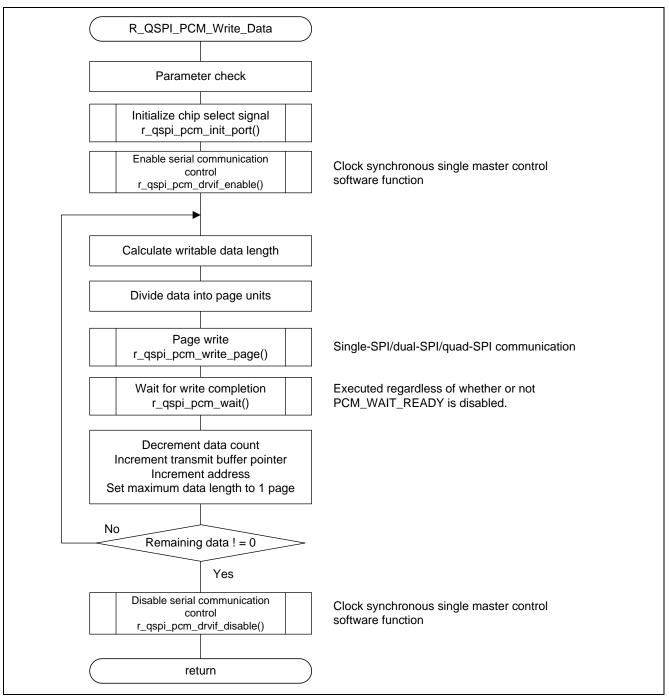
Figure 5.14 Overview of Data Write Processing
