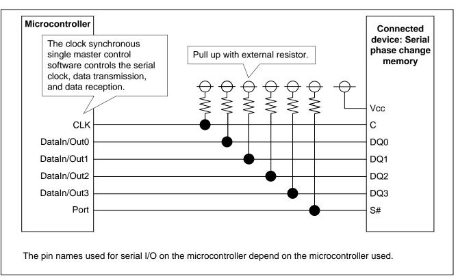
Figure 4.3 MCU and SPI Slave Device Connection Example for Quad-SPI
