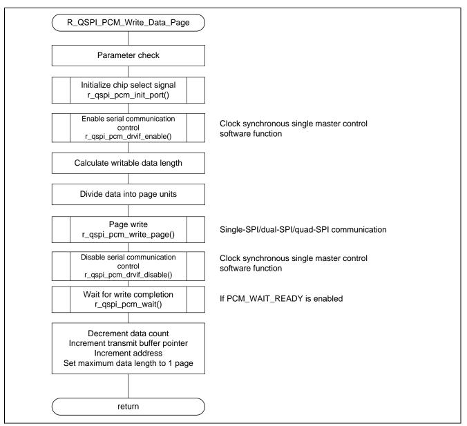
Figure 5.15 Overview of Data Write Processing (for Single-Page Write)
