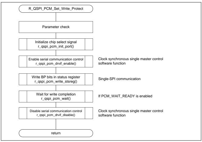
Figure 5.10 Overview of Write Protect Setting Processing
