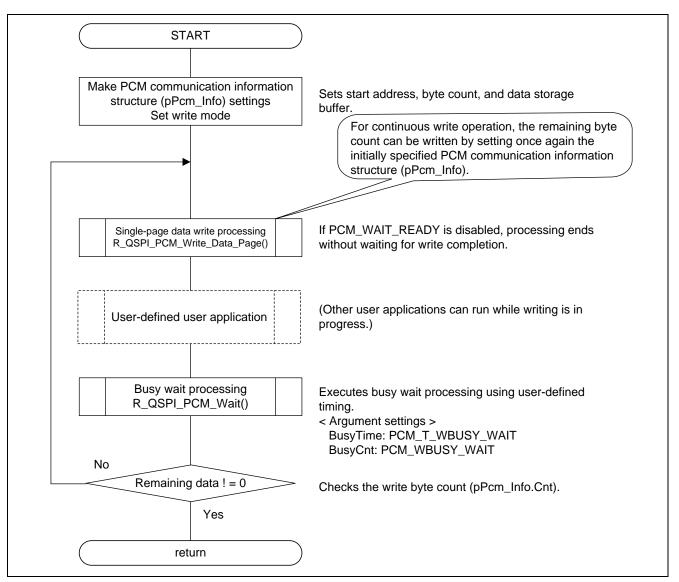
Figure 5.16 Using R\_QSPI\_PCM\_Wait() to Wait for Data Write Processing (for Single-Page Write) Completion
