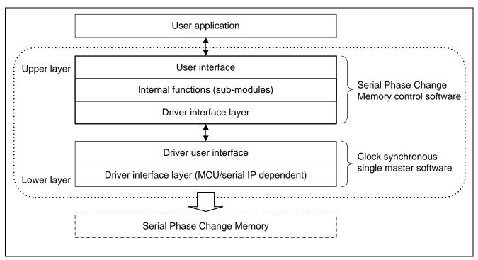
Figure 5.5 Software Configuration
