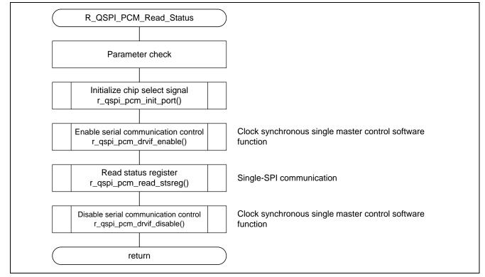
Figure 5.9 Overview of Status Register Read Processing
