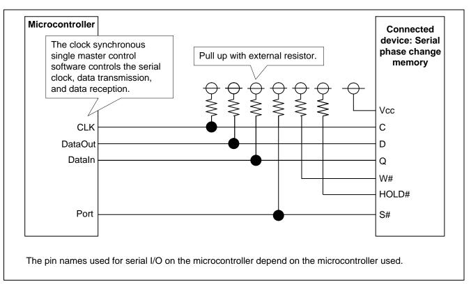
Figure 4.1 MCU and SPI Slave Device Connection Example for Single-SPI
