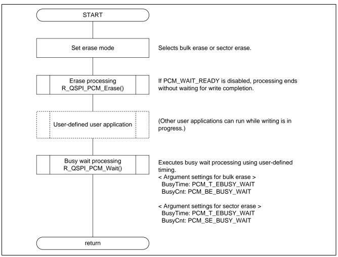
Figure 5.18 Using R\_QSPI\_PCM\_Wait() to Wait for Erase Processing Completion
