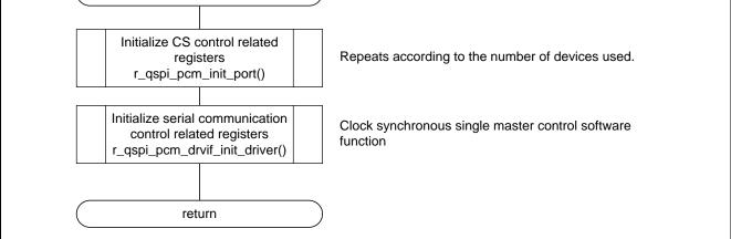
Figure 5.8 Overview of Driver Initialization Processing
