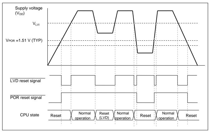
Figure 1.1 Overview of LVD Operation (Reset Mode)
