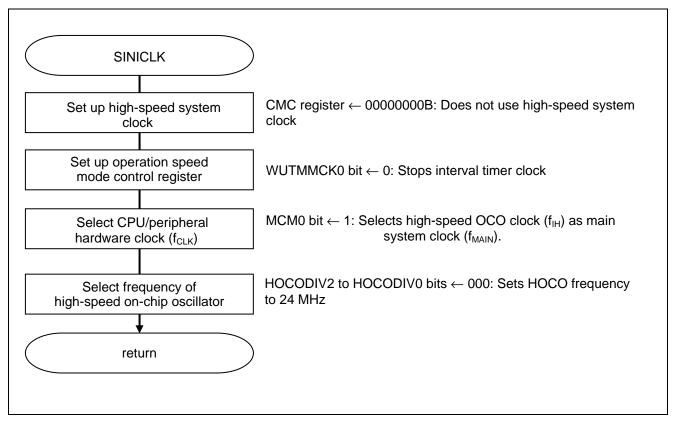
Figure 5.5 Clock Generation Circuit Setup
