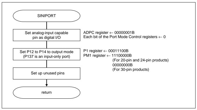
Figure 5.4 I/O Port Setup
