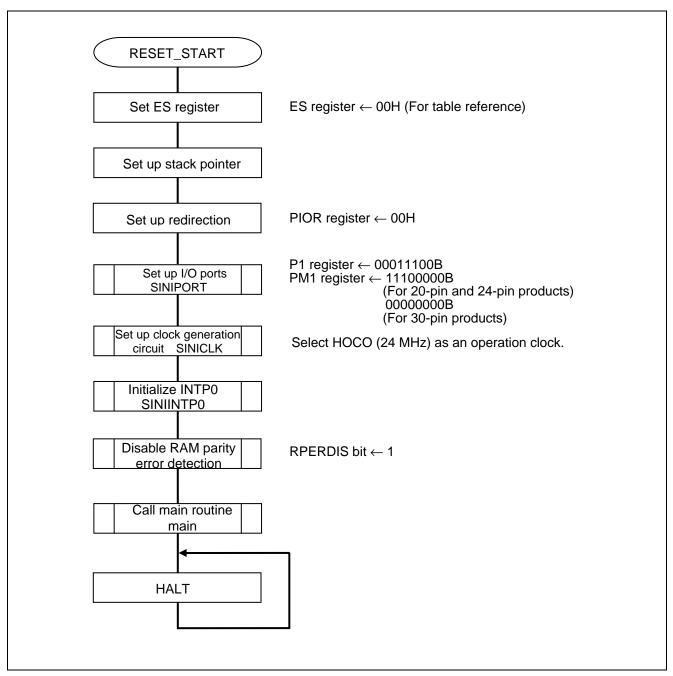
Figure 5.3 CPU Initialization Function
