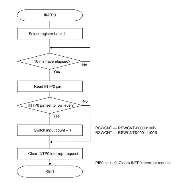
Figure 5.8 INTP0 Interrupt Processing
