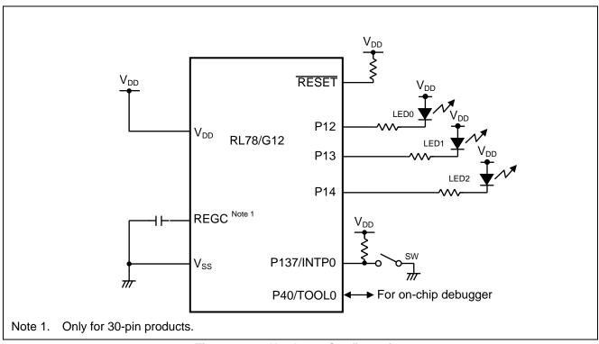
Figure 4.1 Hardware Configuration
