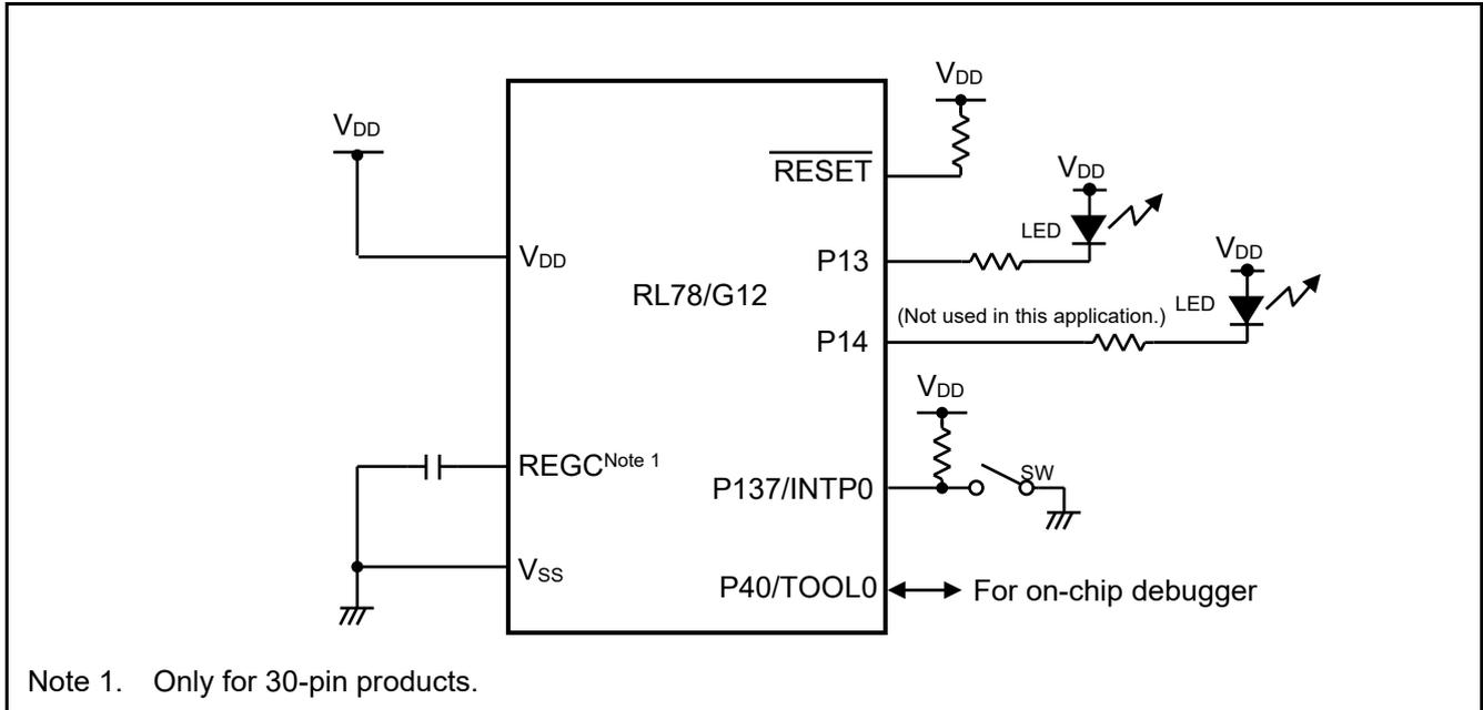
**Figure 4.1 Hardware Configuration**
