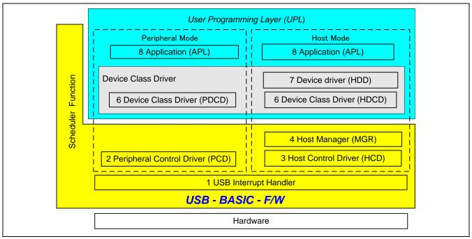
Figure 4.1 Task Configuration of USB-BASIC-F/W
