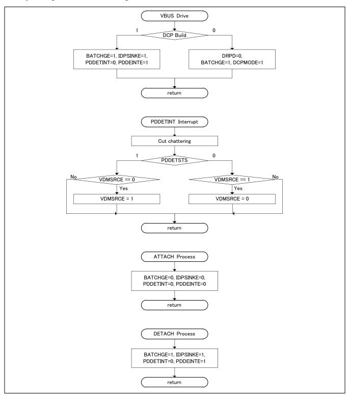
Figure 8.1 HBC processing flow
