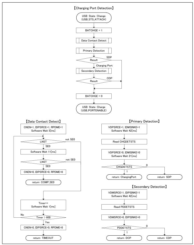
Figure 6.1 PBC processing flow
