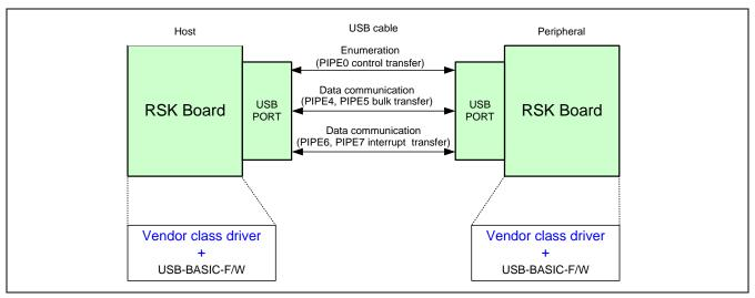
Figure 7.1 Example Full Speed Operating Environment
