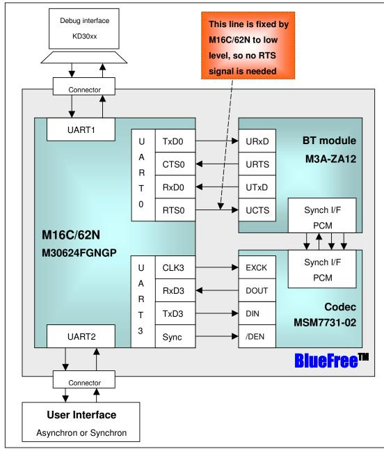
Figure2: Block diagram of BlueFree<sup>™</sup> reference board
