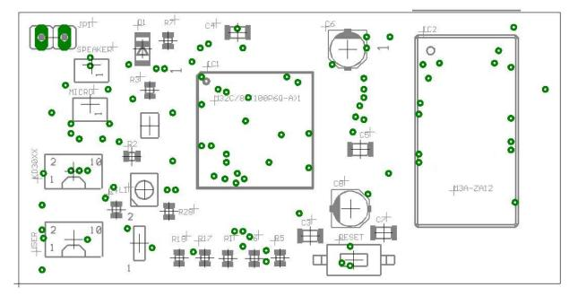
Figure 10: Component placement top layer
