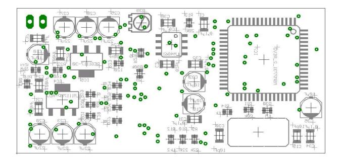
Figure 11: Component placement bottom layer
