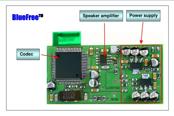
Figure4: Bottom view of BlueFree<sup>™</sup>
