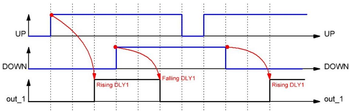
Figure 2: Delay Block Functionality Waveform
