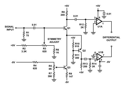
FIGURE 1. SINGLE ENDED TO DIFFERENTIAL TWISTED PAIR DRIVER
