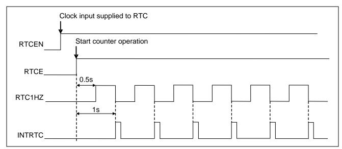
Figure 4.3 Overview of RTC Operation and Interrupts
