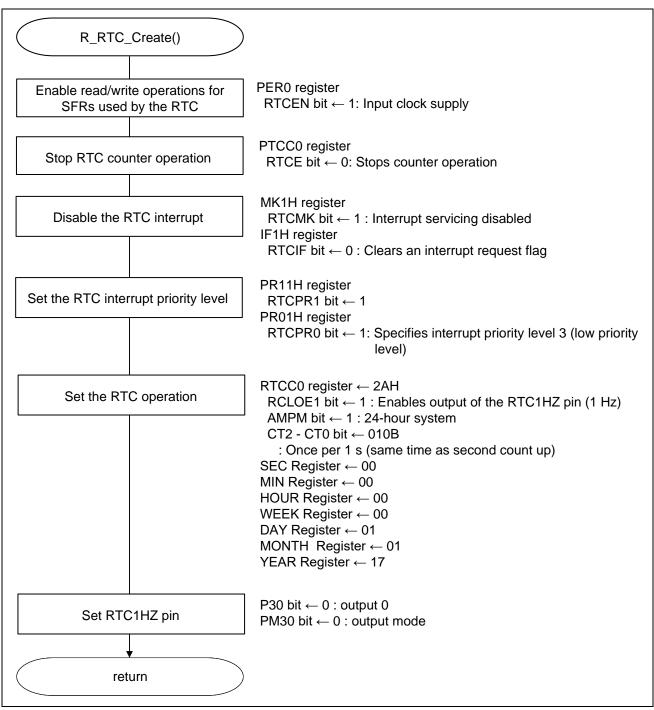
Figure 4.9 Real-Time Clock Setting
