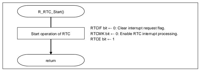
Figure 4.11 Real-Time Clock Operation Start
