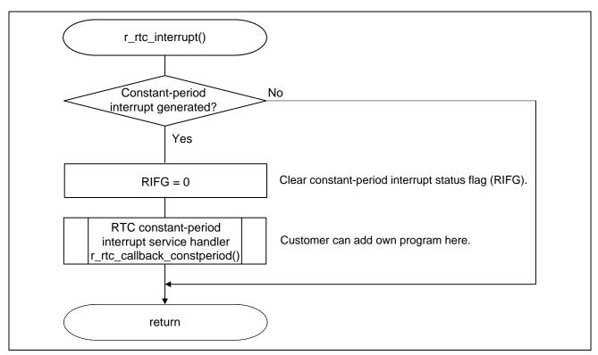
Figure 4.12 INTRTC Interrupt Processing
