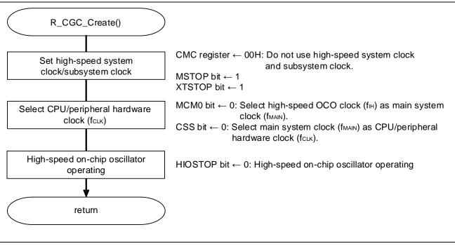
Figure 5.7 CPU Clock Setting
