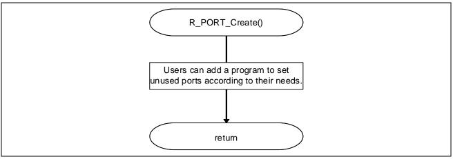
Figure 4.8 I/O Port Setting
