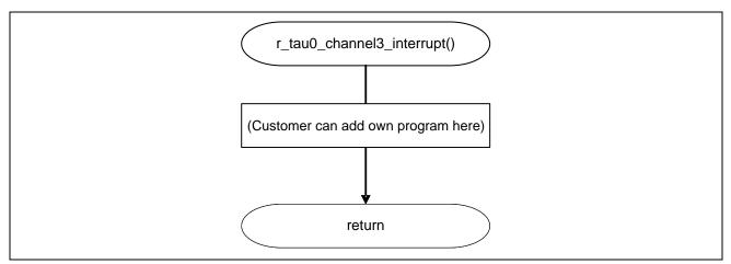
Figure 5.12 INTTM03 Interrupt Processing
