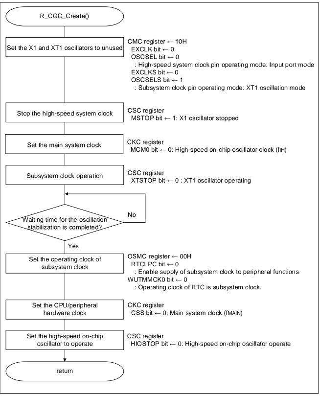
Figure 4.7 CPU Clock Setting
