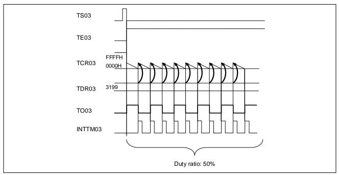
Figure 5.3 Overview of Timer Operation and Interrupts
