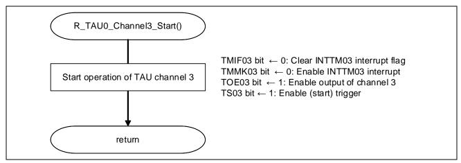
Figure 5.11 Timer Array Unit Operation Start
