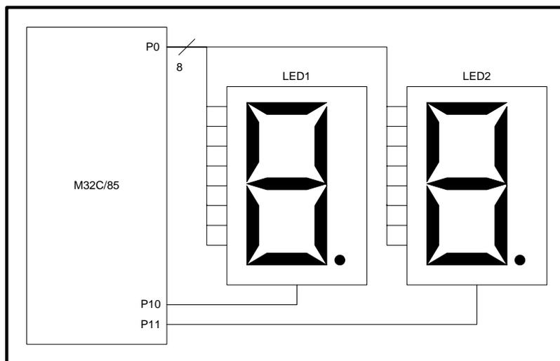
Figure 1. LED Block Diagram (1)
