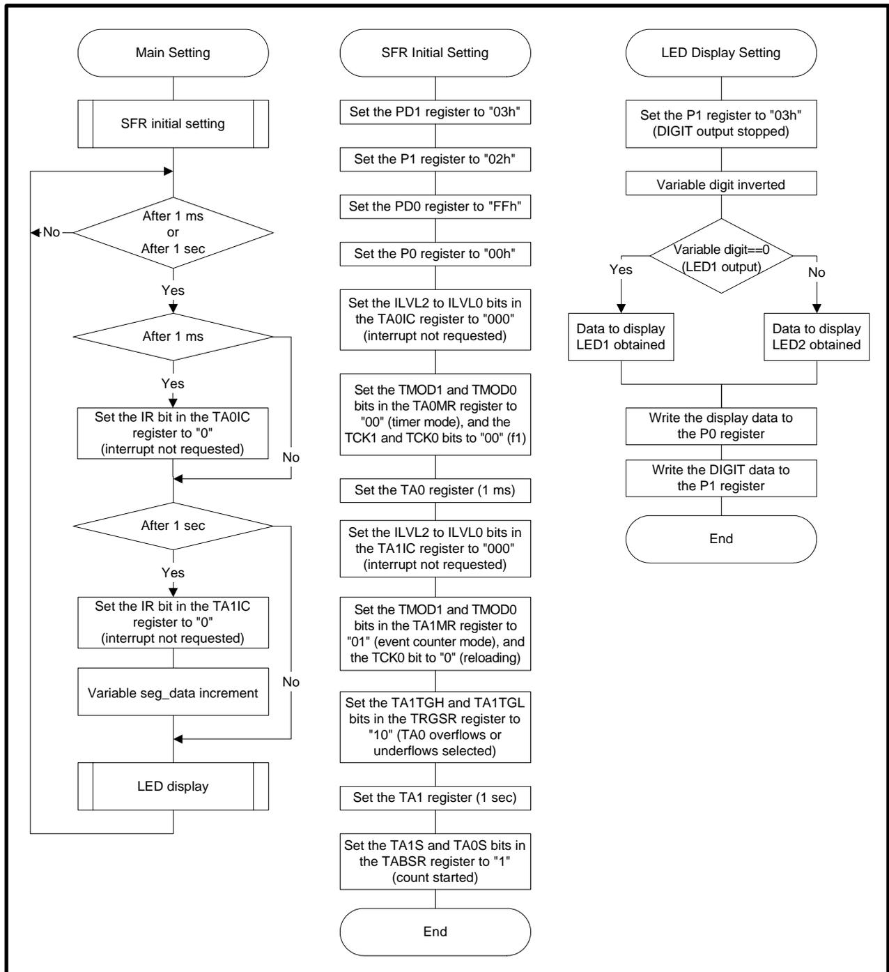
Figure 3. Register Setting Configuration
