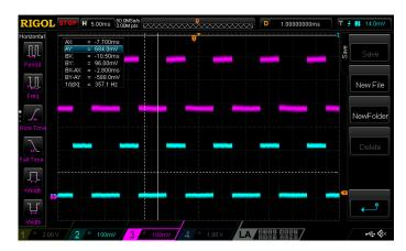
Figure 4 Waveform of voltage across C4
