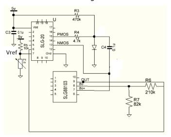
Figure 2 GreenPAK block diagram for the temperature sensing application circuit
