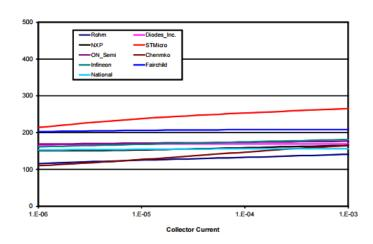
Figure 3.1 Typical Beta Values for 2N3904 Transistors at 23°C (the Microchip lab data)
