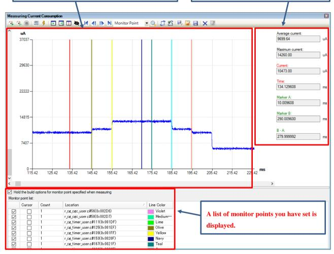
Figure 2 Function of Measuring Current Consumption
