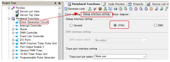
Figure 1 Example of Display when JTAG is Selected
