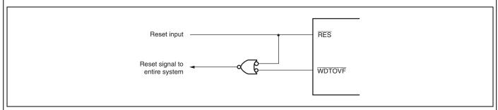
Figure 14.4 Example of System Reset Circuit Using WDTOVF Signal
