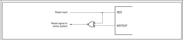
Figure 1 Example of System Reset Circuit Using WDTOVF Signal
