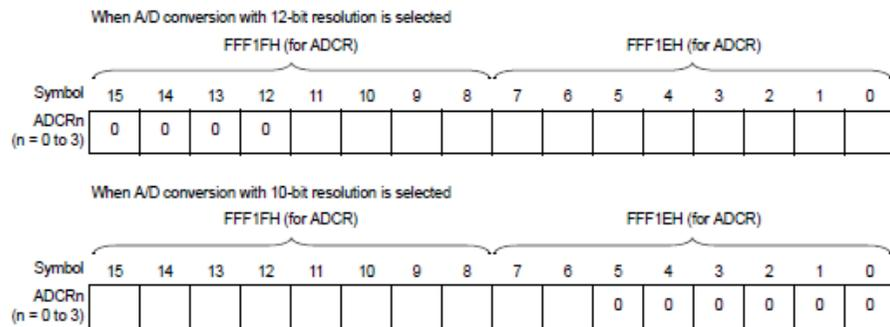
**Note** The contents of the ADCR register are stored in the ADCR0 register.
