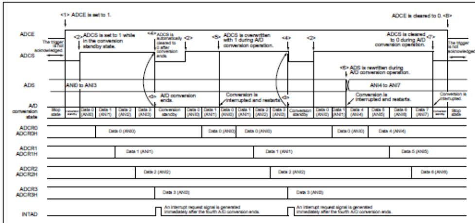
**Caution** When <4>, <5>, or <6> is detected while conversion is in progress, conversion is automatically restarted from the rising edge of the next cycle of the conversion clock (fAD). The conversion time at the first conversion operation restarted is the same as that when there is A/D power supply stabilization wait time in software trigger wait mode or hardware trigger wait mode. (See Table 12 - 3 A/D Conversion Time Selection (3/8) and Table 12 - 3 A/D Conversion Time Selection (4/8).)
