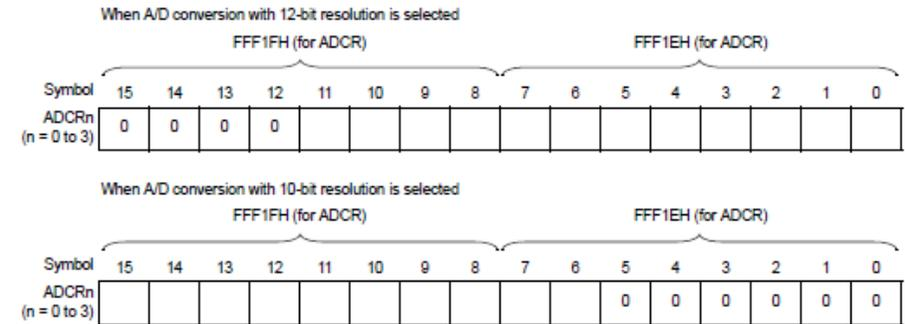
**Note** The contents of the ADCR register are stored in the ADCR0 register.
