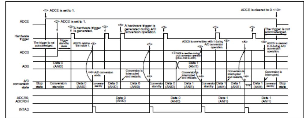
**Caution** When <6>, <7>, or <8> is detected while conversion is in progress, conversion is automatically restarted from the rising edge of the next cycle of the conversion clock (fAD). The conversion time at the first conversion operation restarted is the same as that when there is A/D power supply stabilization wait time in software trigger wait mode or hardware trigger wait mode. (See Table 12 - 3 A/D Conversion Time Selection (3/8) and Table 12 - 3 A/D Conversion Time Selection (4/8).)
