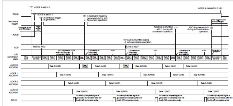
**Caution** When <4>, <5>, or <6> is detected while conversion is in progress, conversion is automatically restarted from the rising edge of the next cycle of the conversion clock (fAD). The conversion time at the first conversion operation restarted is the same as that when there is A/D power supply stabilization wait time in software trigger wait mode or hardware trigger wait mode. (See Table 12 - 3 A/D Conversion Time Selection (3/8) and Table 12 - 3 A/D Conversion Time Selection (4/8).)
