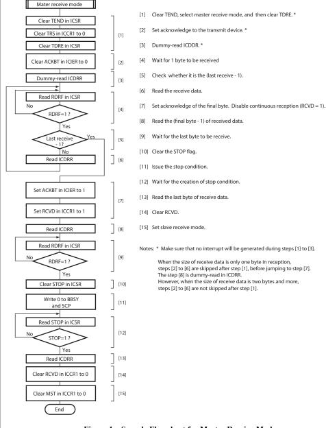
Figure 1 Sample Flowchart for Master Receive Mode
