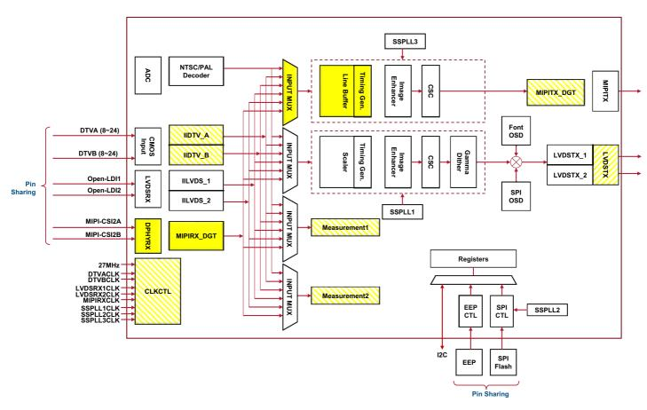
Figure 1. RAA278840 Functional Block Diagram
