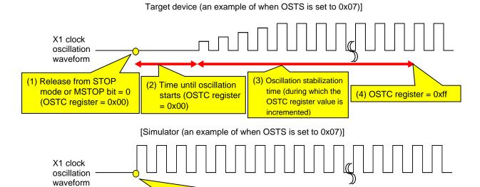
Release from STOP mode or MSTOP bit = 0The OSTC register is set to 0xff at this point. Therefore, pay attention to the code that waits for oscillation stabilization.
