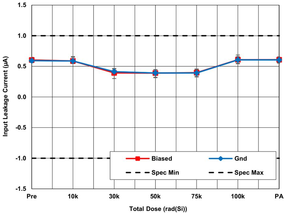
Figure 13. ISL73141SEHMF7 average input leakage current ( $I_{IN}$ ) with  $AV_{CC} = 5V$ ,  $DV_{CC} = 2.5V$ ,  $REF = 4.096V$  as a function of LDR irradiation and anneal. The error bars represent the minimum and maximum measured values. The datasheet limits are  $-1\mu A$  minimum and  $1\mu A$  maximum.
