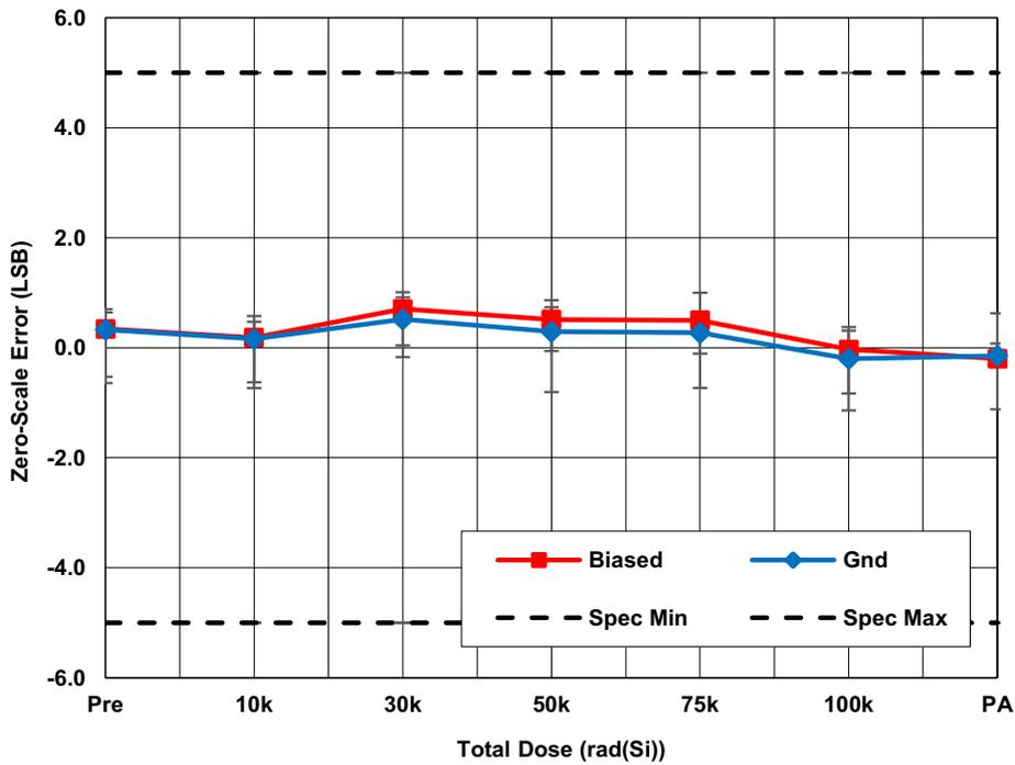
Figure 6. ISL73141SEHMF7 average zero-scale error (VOFF) with  $AV_{CC} = 5V$ ,  $DV_{CC} = 2.5V$ ,  $REF = 4.096V$ ,  $f_{SAMP} = 1Mps$ , and  $A_{IN} = GND$  as a function of LDR irradiation and anneal. The error bars represent the minimum and maximum measured values. The datasheet limits are -5 LSB minimum and 5 LSB maximum.
