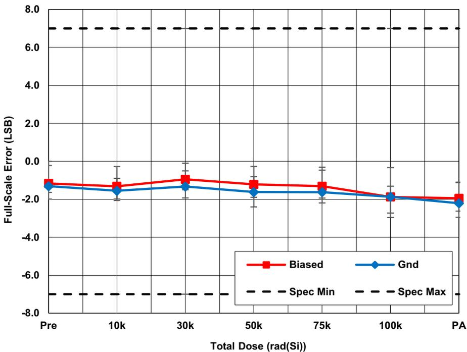
Figure 7. ISL73141SEHMF7 average full-scale error (FSE) with  $AV_{CC} = 5.0V$ ,  $DV_{CC} = 2.5V$ ,  $REF = 4.096V$ ,  $f_{SAMP} = 1Mps$ , and  $A_{IN} = VREF$  as a function of LDR irradiation and anneal. The error bars represent the minimum and maximum measured values. The datasheet limits are -7 LSB minimum and 7 LSB maximum.
