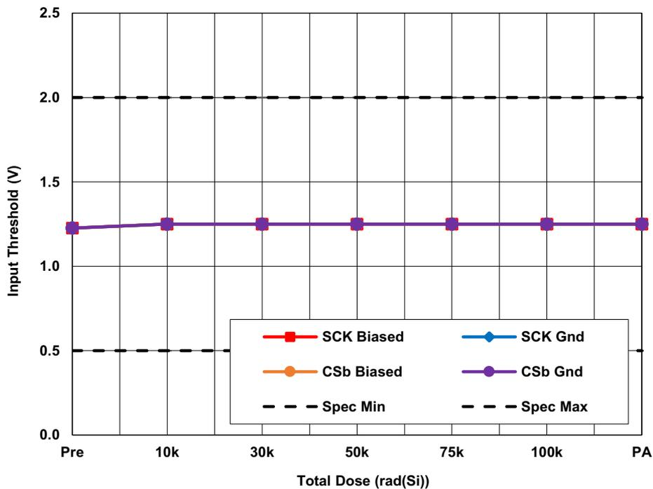
Figure 21. ISL73141SEHMF7 average high-level input ( $V_{IH}$ ) and low level input ( $V_{IL}$ ) with  $AV_{CC} = 5V$ ,  $DV_{CC} = 2.5V$ ,  $REF = 4.096V$  as a function of LDR irradiation and anneal. The error bars (if visible) represent the minimum and maximum measured values. The datasheet limit for  $V_{IH}$  is 2.0V minimum and the datasheet limit for  $V_{IL}$  is 0.5V maximum.
