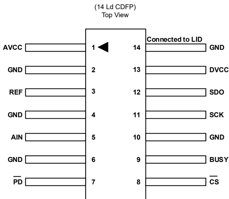
Note: The ESD triangular mark is indicative of Pin #1. It is a part of the device marking and is placed on the lid in the quadrant where Pin #1 is located.
