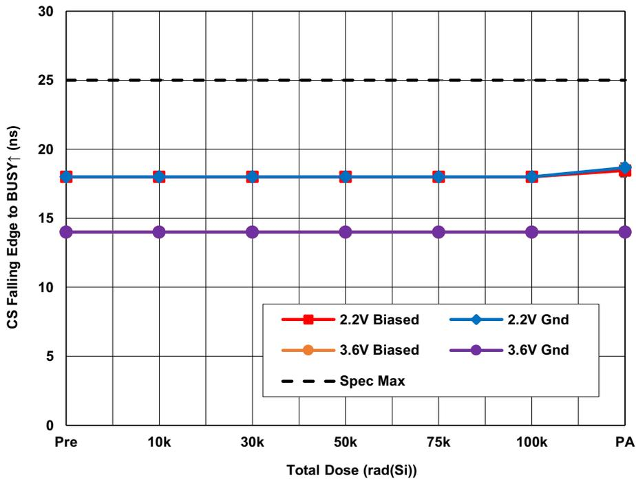
Figure 28. ISL73141SEHMF7 average  $\overline{CS}$  falling edge to BUSY rising edge ( $t_{BUSY_{LH}}$ ) with  $AV_{CC} = 4.5V$ ,  $DV_{CC} = 2.2V$  and  $AV_{CC} = 5.5V$ ,  $DV_{CC} = 3.6V$ ,  $REF = 4.096V$ ,  $f_{SAMP} = 1Msps$ ,  $A_{IN} = -1dbFS$  and  $C_L = 10pF$  as a function of LDR irradiation and anneal. The error bars represent the minimum and maximum measured values. The datasheet limit is 25ns maximum.
