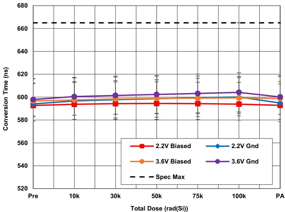
Figure 27. ISL73141SEHMF7 average conversion time ( $t_{CONV}$ ) with  $AV_{CC} = 4.5V$ ,  $DV_{CC} = 2.2V$  and  $AV_{CC} = 5.5V$ ,  $DV_{CC} = 3.6V$ ,  $REF = 4.096V$ ,  $f_{SAMP} = 1Mps$ , and  $A_{IN} = -1dbFS$  as a function of LDR irradiation and anneal. The error bars represent the minimum and maximum measured values. The datasheet limit is  $665ns$  maximum.
