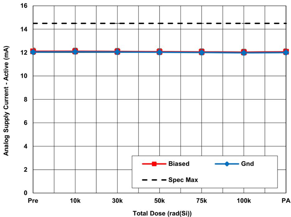
Figure 15. ISL73141SEHMF7 average analog supply current - active ( $I_{AVCC}$ ) with  $AV_{CC} = 5V$ ,  $DV_{CC} = 2.5V$ ,  $REF = 4.096V$ ,  $f_{SAMP} = 1Msps$ , and  $A_{IN} = -1dBFS$  as a function of LDR irradiation and anneal. The error bars represent the minimum and maximum measured values. The datasheet limit is 14.5mA maximum.
