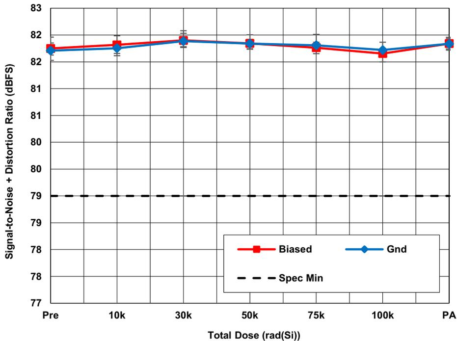
Figure 9. ISL73141SEHMF7 average signal-to-noise + distortion ratio (SINAD) with  $AV_{CC} = 5.0V$ ,  $DV_{CC} = 2.5V$ ,  $REF = 4.096V$ ,  $f_{SAMP} = 105ksps$ , and  $A_{IN} = -1dBFS$  as a function of LDR irradiation and anneal. The error bars represent the minimum and maximum measured values. The datasheet limit is 79dB minimum.
