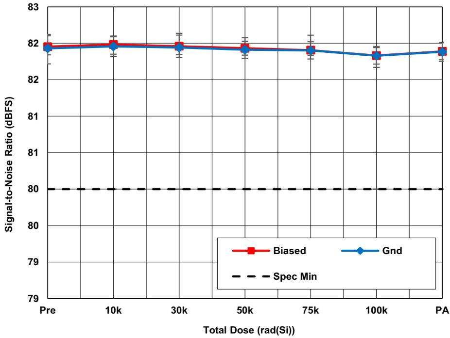
Figure 8. iSL73141SEHMF7 average signal-to-noise ratio (SNR) with  $AV_{CC} = 5.0V$ ,  $DV_{CC} = 2.5V$ ,  $REF = 4.096V$ ,  $f_{SAMP} = 105ksps$  and  $A_{IN} = -1dBFS$  as a function of LDR irradiation and anneal. The error bars represent the minimum and maximum measured values. The datasheet limit is 80dB minimum.
