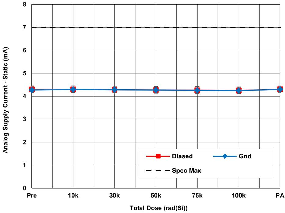
Figure 16. ISL73141SEHMF7 average analog supply current - static ( $I_{STATIC}$ ) with  $AV_{CC} = 5V$ ,  $DV_{CC} = 2.5V$ ,  $REF = 4.096V$ , and  $CS = DV_{CC}$  as a function of LDR irradiation and anneal. The error bars represent the minimum and maximum measured values. The datasheet limit is 7mA maximum.
