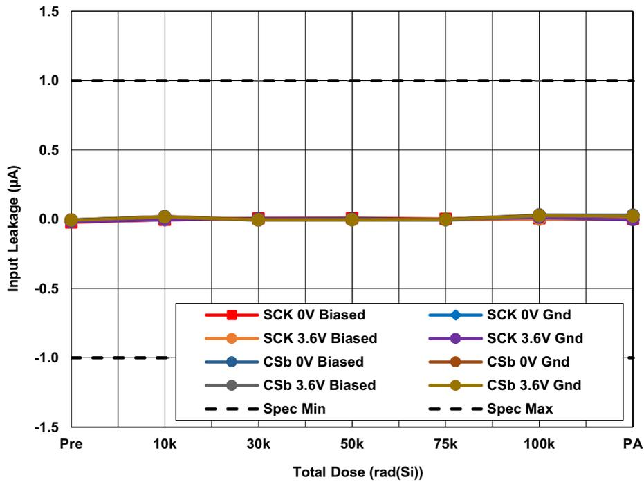
Figure 22. ISL73141SEHMF7 average input leakage current ( $I_{IN}$ ) on SCK and  $\overline{CS}$  with  $AV_{CC} = 5V$ ,  $DV_{CC} = 2.5V$ ,  $REF = 4.096V$  and  $V_{IN} = 0V$  and  $5V$  as a function of LDR irradiation and anneal. The error bars (if visible) represent the minimum and maximum measured values. The datasheet limits are  $-1\mu A$  minimum and  $1\mu A$  maximum.
