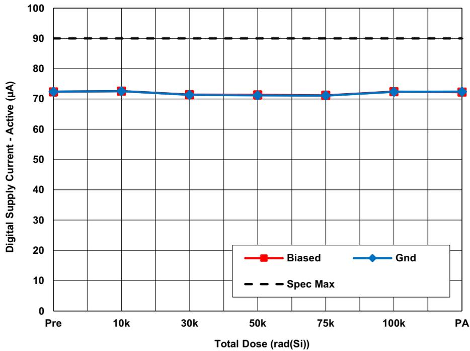
Figure 18. ISL73141SEHMF7 average digital supply current - active ( $I_{DVCC}$ ) with  $AV_{CC} = 5V$ ,  $DV_{CC} = 2.5V$ ,  $REF = 4.096V$ ,  $f_{SCK} = 50MHz$ , and  $C_L = 10pF$  as a function of LDR irradiation and anneal. The error bars represent the minimum and maximum measured values. The datasheet limit is  $90\mu A$  maximum.
