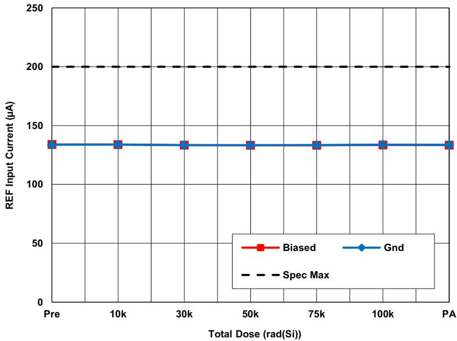
Figure 14. ISL73141SEHMF7 average REF input current ( $I_{REF}$ ) with  $AV_{CC} = 5V$ ,  $DV_{CC} = 2.5V$ ,  $REF = 4.096V$  as a function of LDR irradiation and anneal. The error bars represent the minimum and maximum measured values. The datasheet limit is 200µA maximum.
