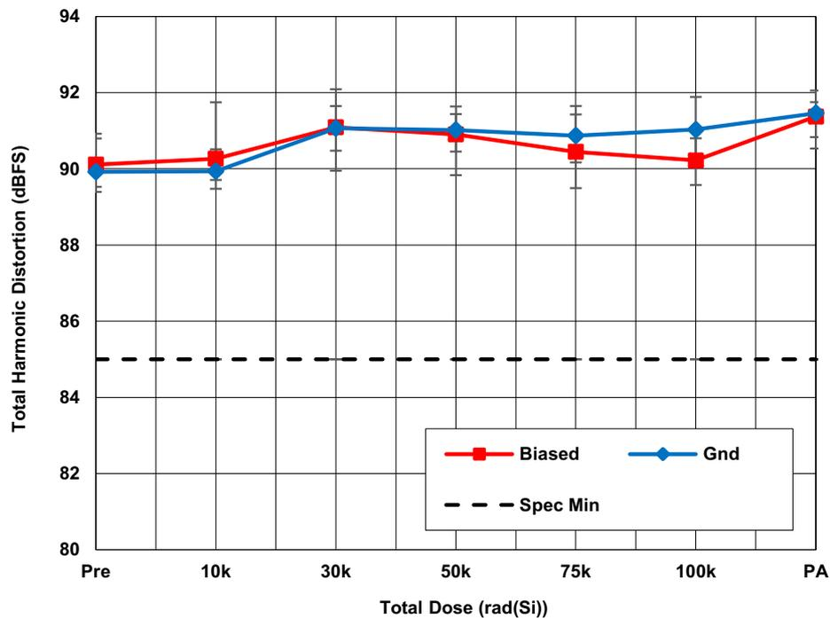
Figure 11. ISL73141SEHMF7 average total harmonic distortion (THD) with  $AV_{CC} = 5.0V$ ,  $DV_{CC} = 2.5V$ ,  $REF = 4.096V$ ,  $f_{SAMP} = 105ksps$  (first five harmonics), and  $A_{IN} = -1dBFS$  as a function of LDR irradiation and anneal. The error bars represent the minimum and maximum measured values. The datasheet limit is 85dB minimum.
