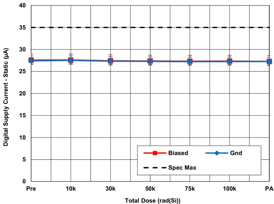
Figure 19. ISL73141SEHMF7 average digital supply current - static ( $I_{STDVCC}$ ) with  $AV_{CC} = 5V$ ,  $DV_{CC} = 2.5V$ ,  $REF = 4.096V$ , and  $CS = DV_{CC}$  as a function of LDR irradiation and anneal. The error bars represent the minimum and maximum measured values. The datasheet limit is  $35\mu A$  maximum.
