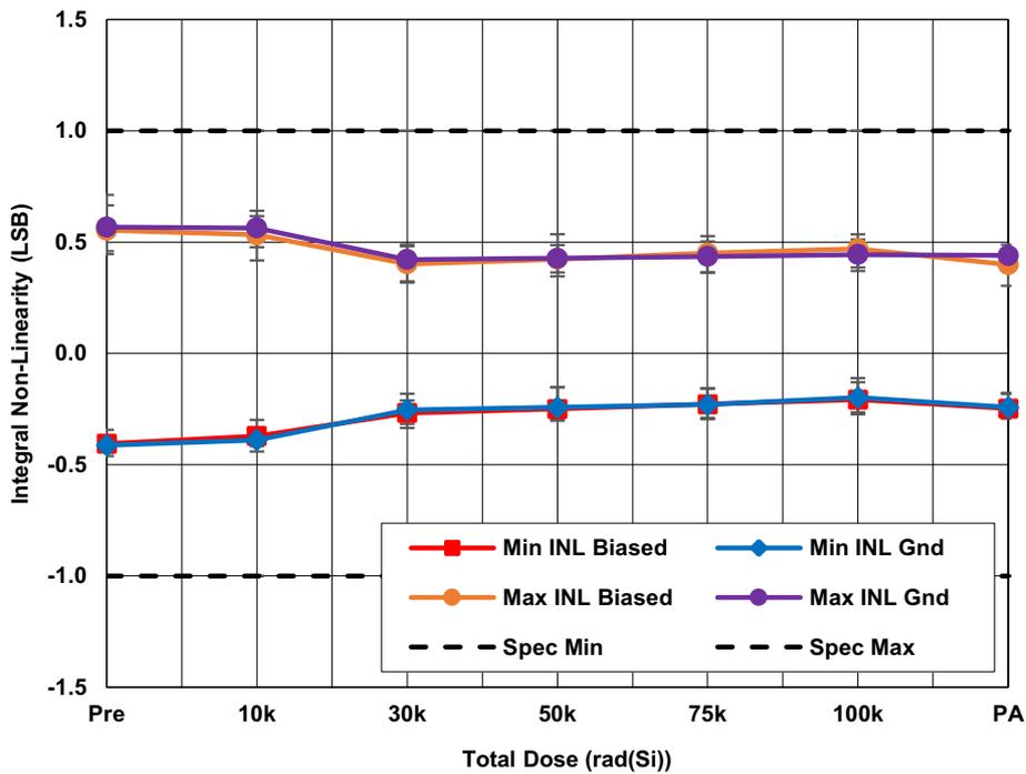
Figure 4. ISL73141SEHMF7 average minimum and maximum integral non-linearity (INL) with  $AV_{CC} = 5V$ ,  $DV_{CC} = 2.5V$ ,  $REF = 4.096V$ ,  $f_{SAMP} = 1Mpsps$ , and  $A_{IN} =$  full-scale sine wave as a function of LDR irradiation and anneal. The error bars represent the minimum and maximum measured values. The datasheet limits are -1 LSB minimum and 1 LSB maximum.
