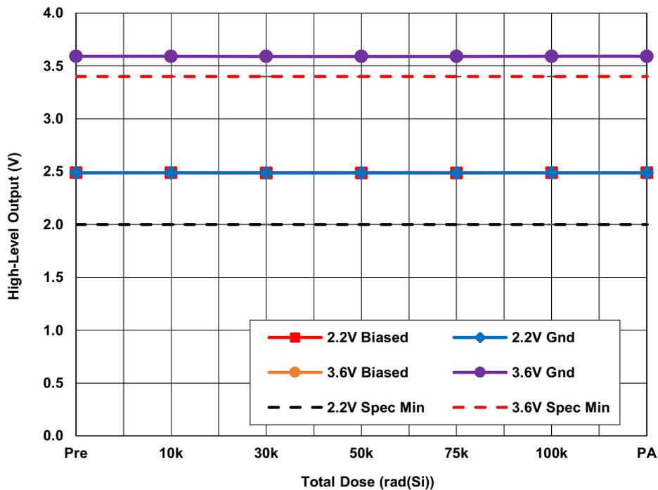
Figure 23. ISL73141SEHMF7 average high-level output ( $V_{OH}$ ) with  $AV_{CC} = 5V$ ,  $DV_{CC} = 2.2V$  and  $3.6V$ ,  $REF = 4.096V$  and  $I_O = -500\mu A$  as a function of LDR irradiation and anneal. The error bars (if visible) represent the minimum and maximum measured values. The datasheet limits are  $2.0V$  minimum for  $DV_{CC} = 2.2V$  and  $3.4V$  minimum for  $DV_{CC} = 3.6V$ .
