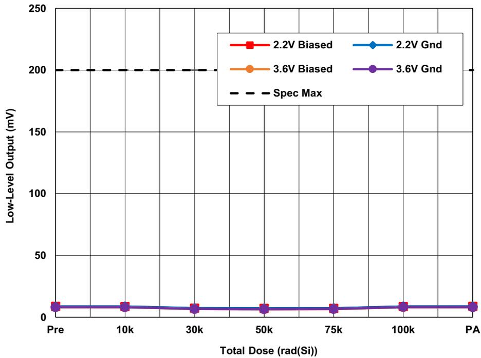
Figure 24. ISL73141SEHMF7 average low-level output ( $V_{OL}$ ) with  $AV_{CC} = 5V$ ,  $DV_{CC} = 2.5V$  and  $3.6V$ ,  $REF = 4.096V$ , and  $I_O = 500\mu A$  as a function of LDR irradiation and anneal. The error bars (if visible) represent the minimum and maximum measured values. The datasheet limit is 200mV maximum.
