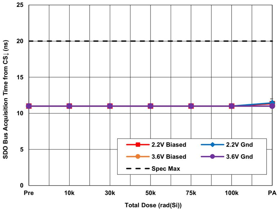
Figure 31. ISL73141SEHMF7 average SDO bus acquisition time from  $\overline{CS}$  falling edge ( $t_{DCSLSDOL}$ ) with  $AV_{CC} = 4.5V$ ,  $DV_{CC} = 2.2V$  and  $AV_{CC} = 5.5V$ ,  $DV_{CC} = 3.6V$ ,  $REF = 4.096V$ ,  $f_{SAMP} = 1Msps$ ,  $A_{IN} = -1dbFS$  and  $C_L = 10pF$  as a function of LDR irradiation and anneal. The error bars represent the minimum and maximum measured values. The datasheet limit is 20ns maximum.
