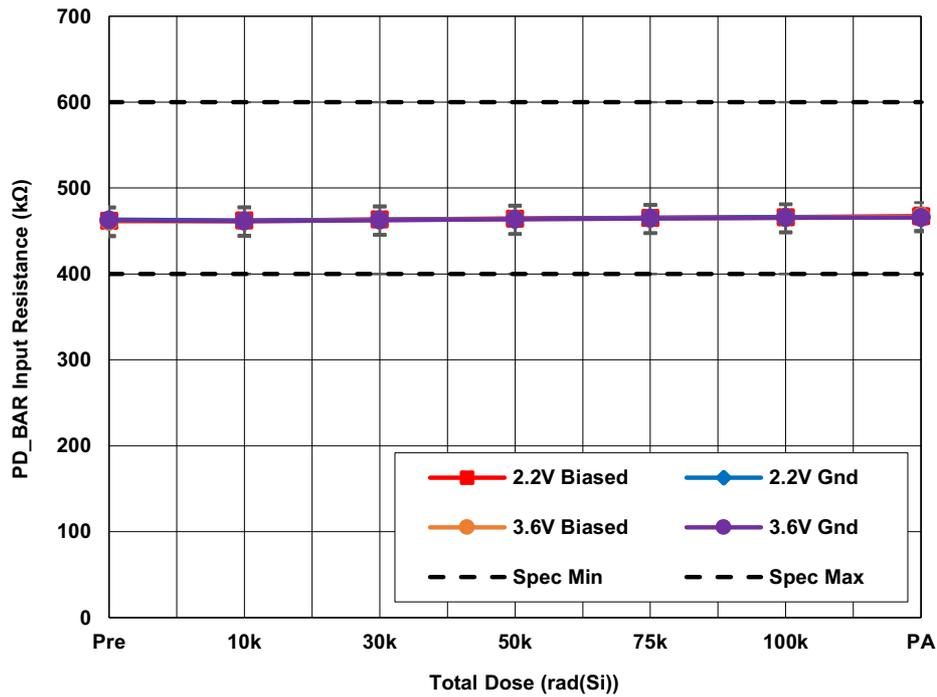
Figure 26. ISL73141SEHMF7 average  $\overline{R_{INPDL}}$  with  $AV_{CC} = 5V$ ,  $DV_{CC} = 2.2V$  and  $3.6V$  and  $REF = 4.096V$  as a function of LDR irradiation and anneal. The error bars represent the minimum and maximum measured values. The datasheet limits are  $400k\Omega$  minimum and  $600k\Omega$  maximum.
