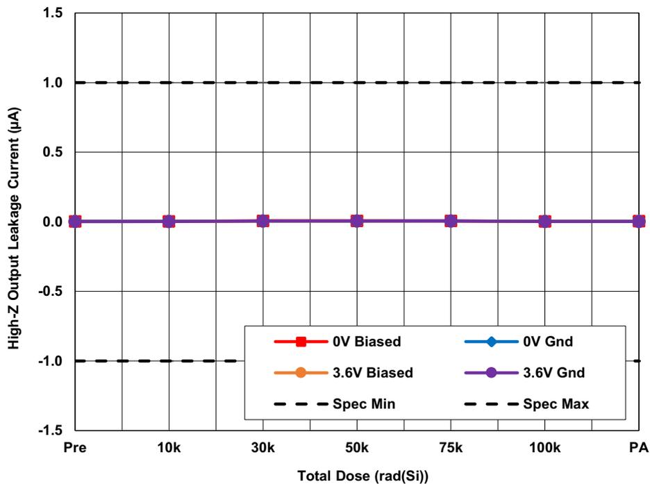
Figure 25. ISL73141SEHMF7 average output leakage current ( $I_{OZ}$ ) with  $AV_{CC} = 5V$ ,  $DV_{CC} = 3.6V$ ,  $REF = 4.096V$ , as a function of LDR irradiation and anneal. The error bars (if visible) represent the minimum and maximum measured values. The datasheet limits are  $-1\mu A$  minimum and  $1\mu A$  maximum.
