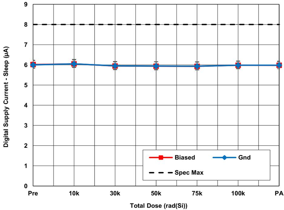
Figure 20. ISL73141SEHMF7 average digital supply current - sleep ( $I_{SLDVCC}$ ) with  $AV_{CC} = 5V$ ,  $DV_{CC} = 2.5V$ ,  $REF = 4.096V$ ,  $PD = GND$  as a function of LDR irradiation and anneal. The error bars represent the minimum and maximum measured values. The datasheet limit is 8µA maximum.
