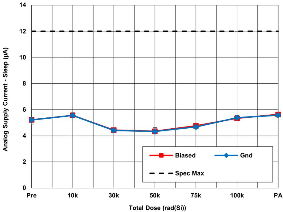
Figure 17. ISL73141SEHMF7 average analog supply current - sleep ( $I_{SLAVCC}$ ) with  $AV_{CC} = 5V$ ,  $DV_{CC} = 2.5V$ ,  $REF = 4.096V$ , and  $PD = GND$  as a function of LDR irradiation and anneal. The error bars represent the minimum and maximum measured values. The datasheet limit is 12 $\mu A$  maximum.
