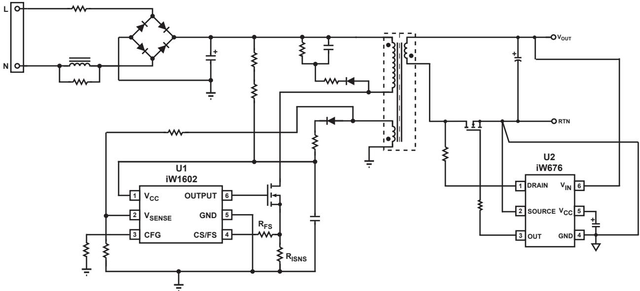
**Figure 3.2 : iW676 Typical Application Circuit Using iW1602 as the Primary-Side Controller (Achieving < 30mW No-Load Power Consumption in 5V, 2.5A Adapter Designs with Fast Dynamic Load Response, and Supporting Constant Current Operation at Low System Output)**
