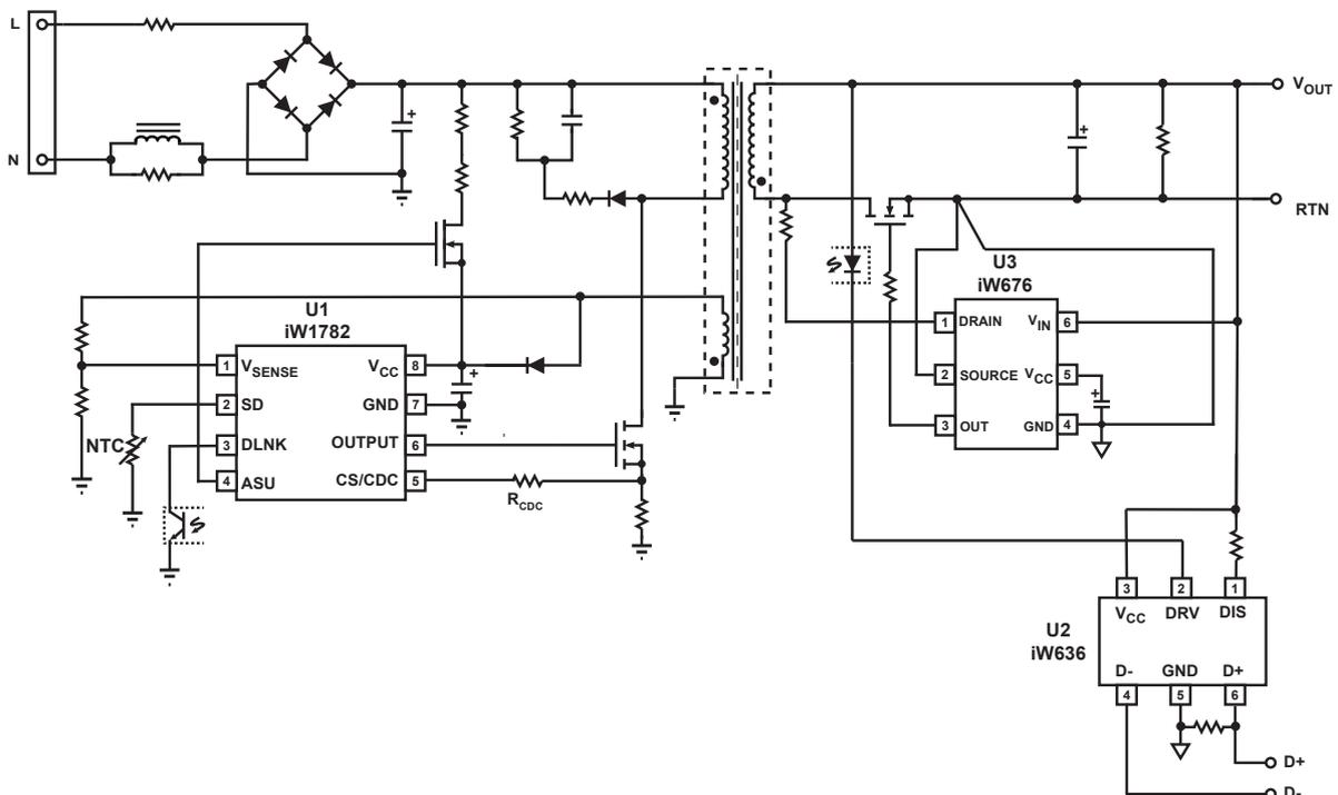
**Figure 3.3 : iW676 Typical Application Circuit for Multi-Level Output Voltage and Current (Using iW1782 as Primary-Side Controller and iW636 as Secondary-Side Controller for Qualcomm® Quick Charge™ 3.0) (Achieving < 20mW No-Load Power Consumption)**
