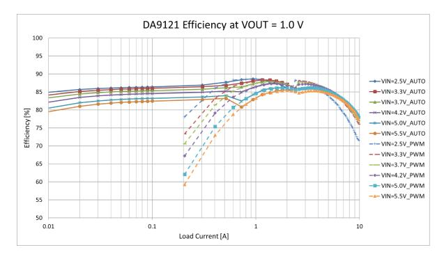
DA9121 operates as a dual-phase buck converter, delivering up to 10 A output current. The output voltage is programmable from 0.3 V to 1.9 V in 10 mV increments. The input voltage range of 2.5 V to 5.5 V makes it suitable for a wide variety of low-voltage systems, including all Li-lon battery powered applications. To guarantee the highest accuracy and to support multiple PCB routing scenarios without loss of performance, a remote differential sensing capability is implemented.
