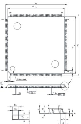
24x24mm 176pin LQFP package drawing (Current)
