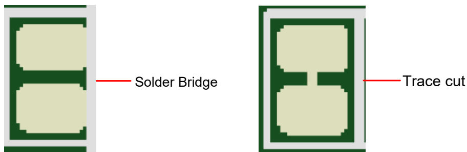
Figure 6-1 Solder Bridge and Trace Cut
