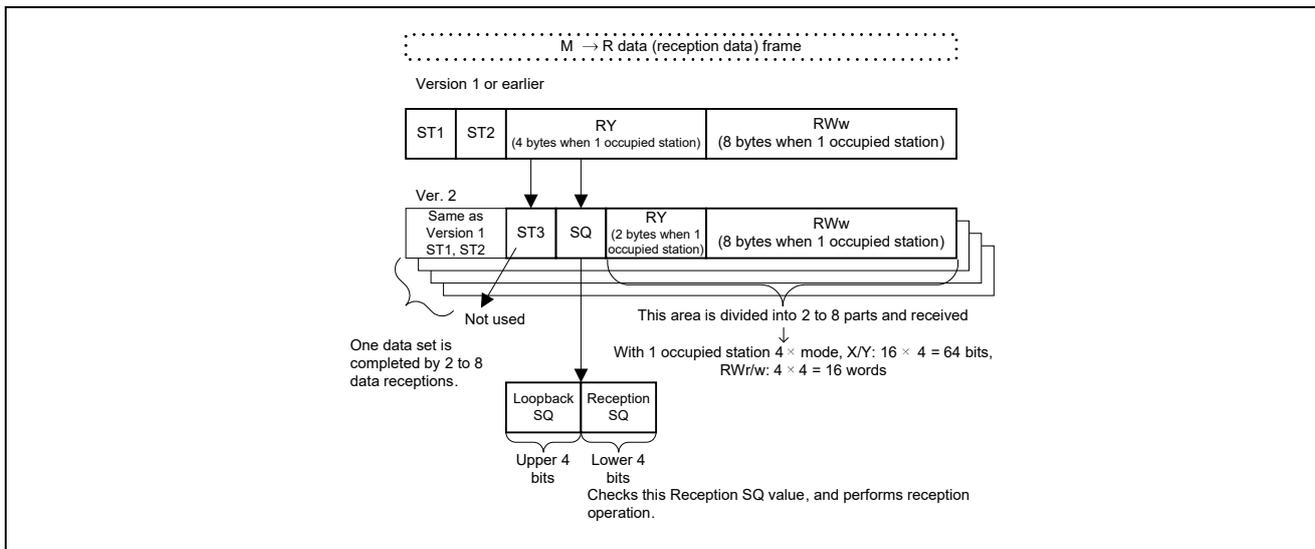
Figure 11.3 Details of SQ Value (M → R Data)
