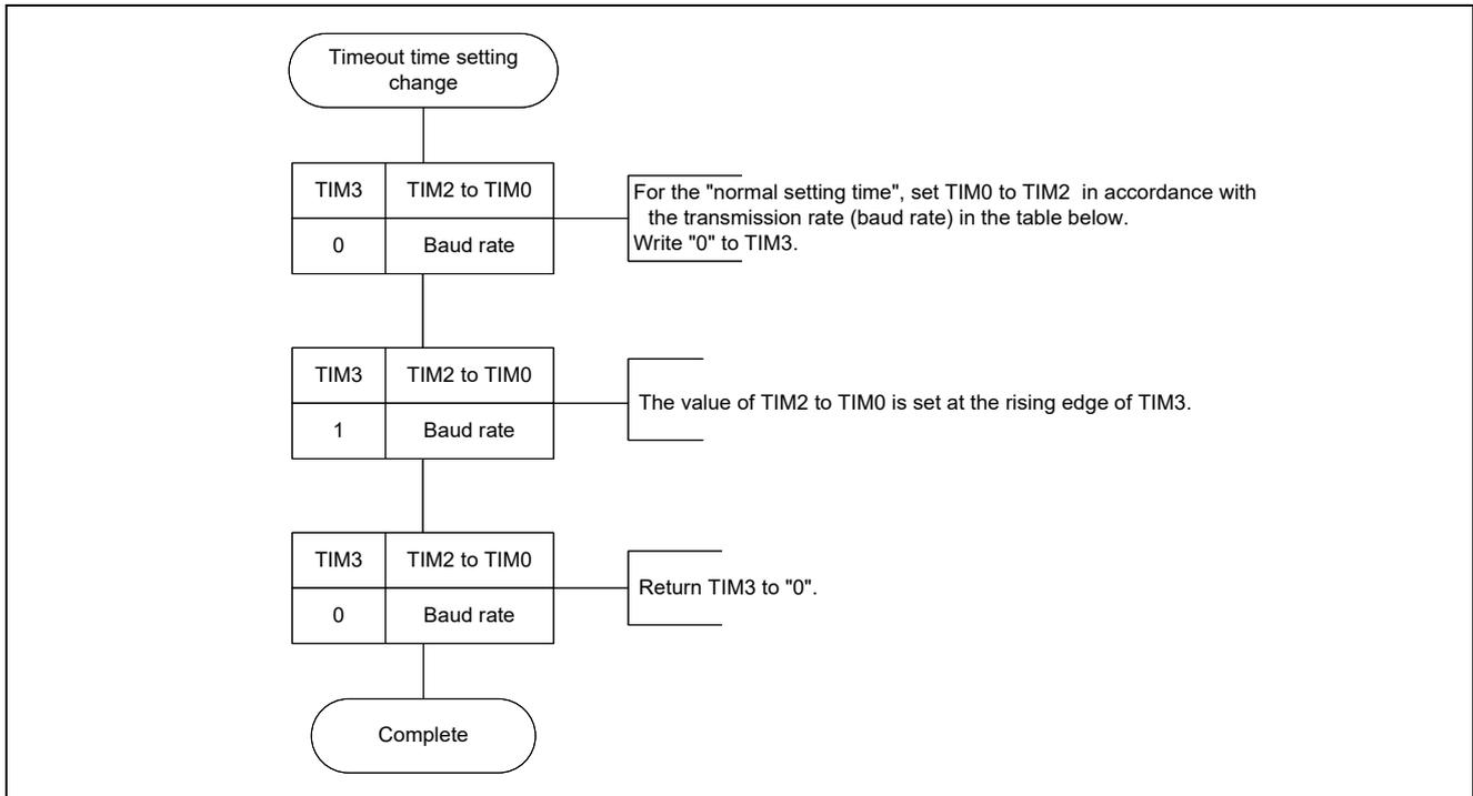
Figure9.8 Normal Setting Time → Initial Setting Time
