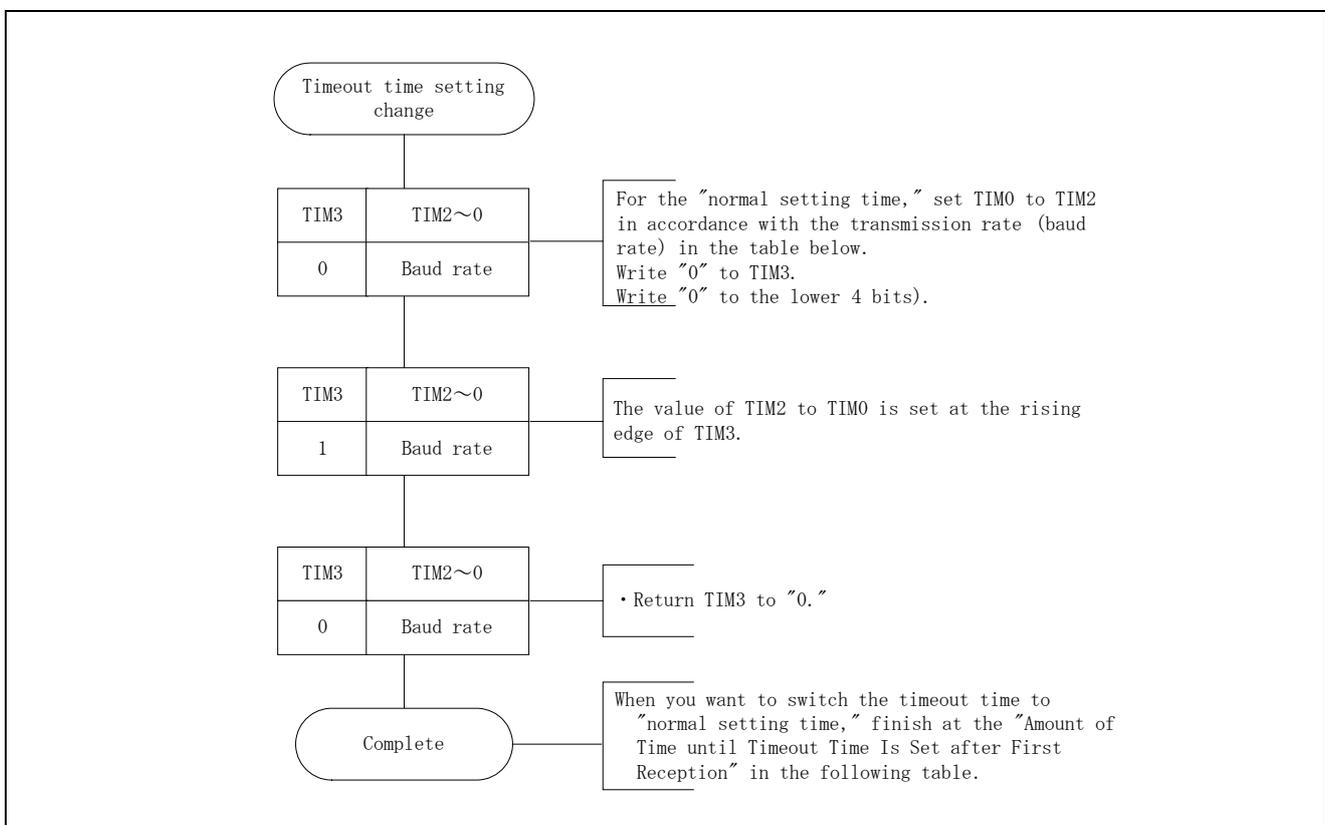
Figure 9.7 Initial Setting Time → Normal Setting Time
