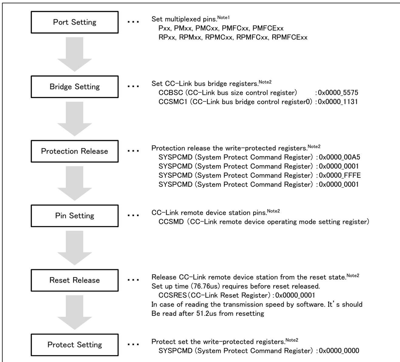
Figure 4.1 How to R-IN32 Series Initialization
