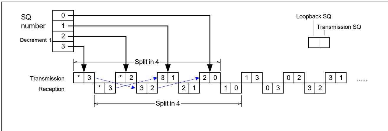
Figure 11.5 Details of SQ Value (Loopback)
