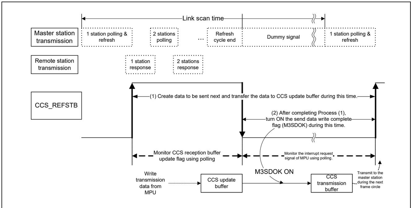
Figure 13.1 Link Scan Time and CCS\_REFSTB Signal Change
