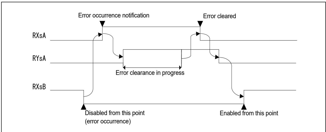
Figure 10.5 RXsA/RYsA (Error Status / Reset Request Flag)
