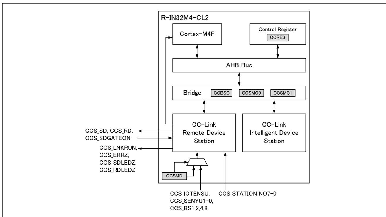
Figure 5.2 R-IN32M4-CL2 CC-Link Remote Device Station Peripheral Architecture
