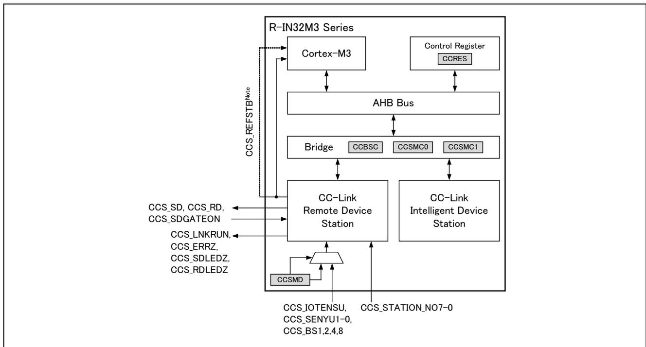
Figure 5.1 R-IN32M3 Series CC-Link Remote Device Station Peripheral Architecture
