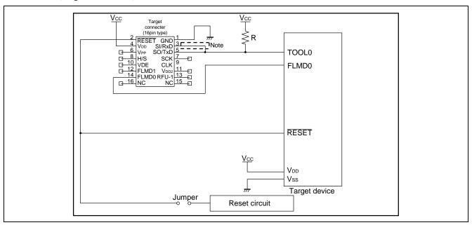
Figure 8.6 Circuit Example for 78K0R (Single-wire UART)
