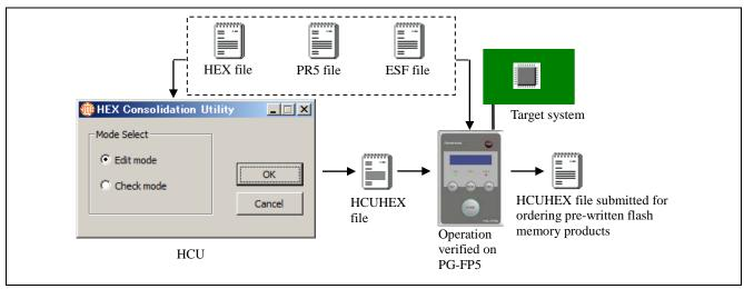
Figure 1.2 PG-FP5 Connection Diagram
