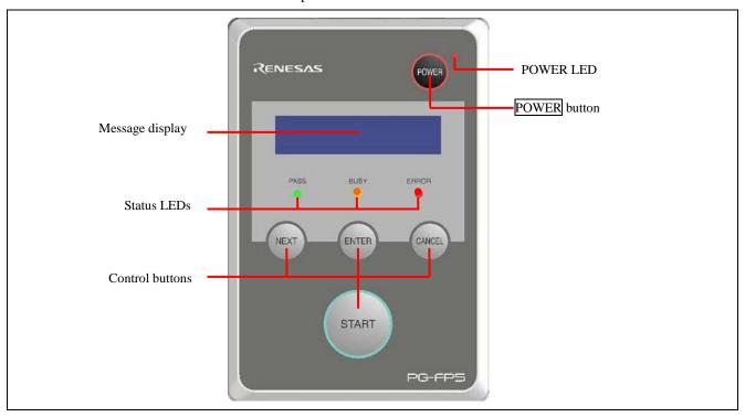
Figure 2.2 FP5 Top View < Control Panel>
