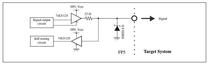
Figure 9.4 FLMD0/IO0/FPMD0, FLMD1, RFU-1/IO1/FPMD1, and VDE/IO2/FPMD2 Pins
