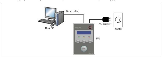
Figure 6.1 **System Connections**
