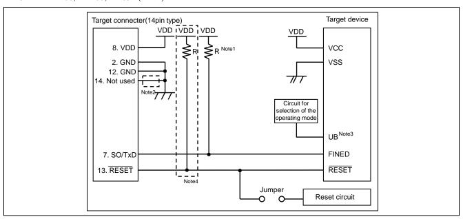
Figure 8.15 Circuit Example for RX100, RX200, RX65x (FINE)
