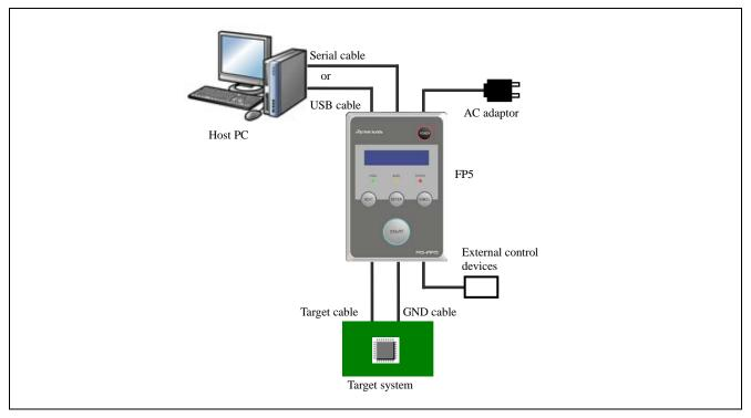
Figure 2.1 FP5 System Configuration
