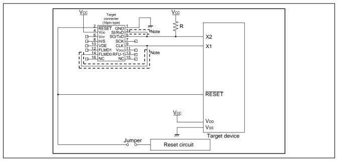
Figure 8.5 Circuit Example for 78K0S (Single-wire UART)
