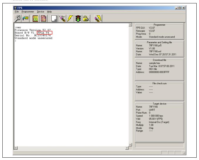
Figure 3.11 Version Confirmation After FPGA Update Is Finished
