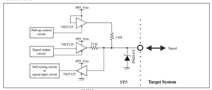
Figure 9.1 SO/TxD/IO3/FPDR/FPMD3, RESET and SCK/IO4/FPCK/FPMD4 Pins
