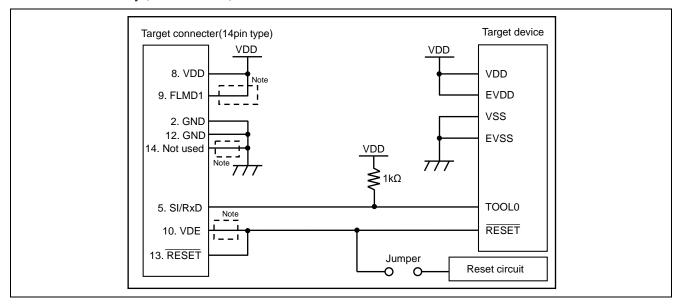
Figure 8.11 Circuit Example for RL78 Family (VDD = EVDD)
