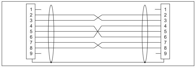
Figure 7.5 **Serial Cable Connection**
