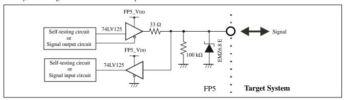
Figure 9.2 SI/RxD/FPDT and H/S Pins
