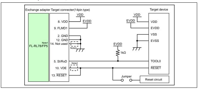
Figure 8.12 Circuit Example for RL78 Family (VDD ≠ EVDD)
