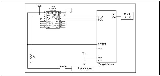
Figure 8.7 Circuit Example for I<sup>2</sup>C
