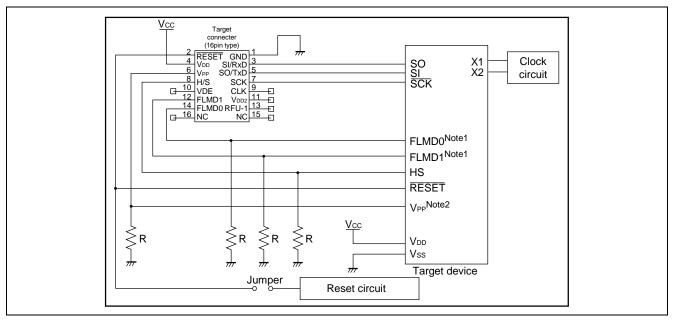
Figure 8.1 78K, V850 (SIO-H/S) Circuit Example
