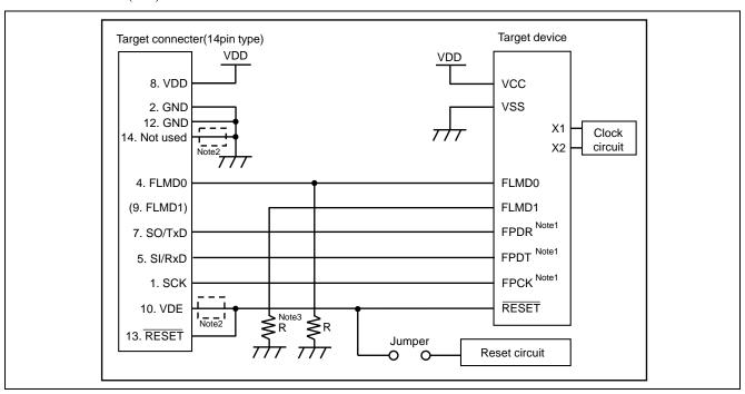
Figure 8.10 Circuit Example for V850E2 (CSI)
