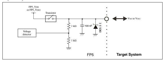
Figure 9.5  $V_{DD}$  and  $V_{DD2}$  Pins
