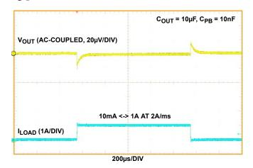
FIGURE 13. LOAD TRANSIENT RESPONSE
