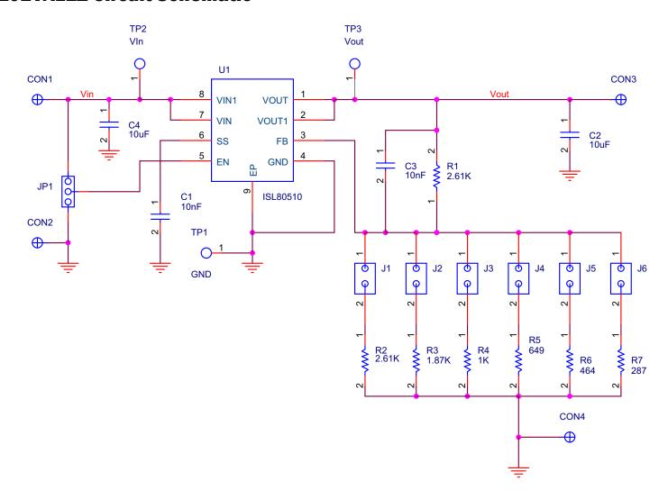
FIGURE 4. ISL80510EVAL1Z SCHEMATIC
