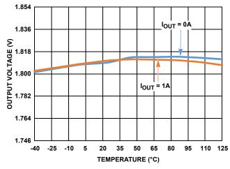
FIGURE 8. OUTPUT VOLTAGE vs TEMPERATURE
