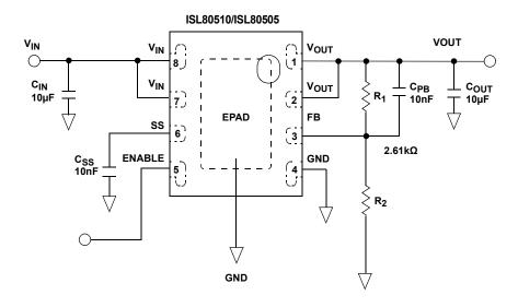
FIGURE 1. ISL80510EVAL1Z BLOCK DIAGRAM
