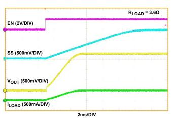
FIGURE 12. ENABLE START-UP (C<sub>SS</sub> = 10nF)
