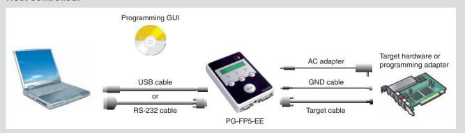
In this mode, the programmer is controlled by a host PC via USB or RS-232 cable.
