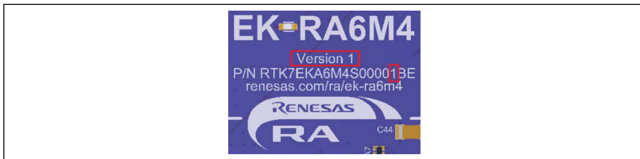
Figure 3. Identification of the Kit Version Number on the EK-RA6M4 Board
