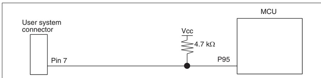
**Figure 4.4 Connection of Emulator and Pin P95**
