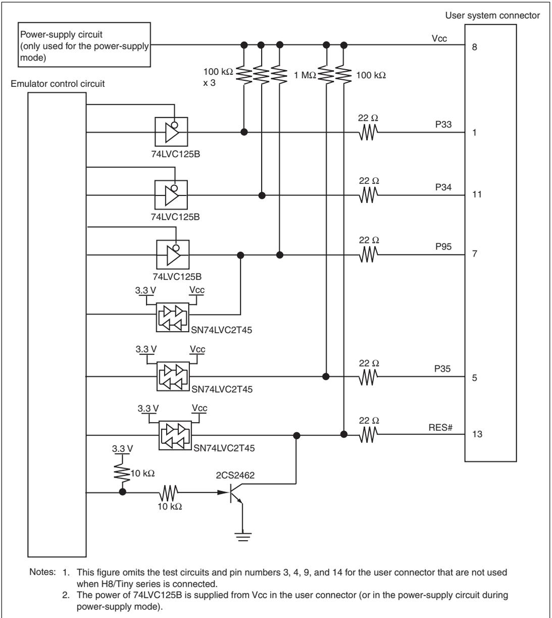
**Figure 4.7 Interface Circuit in the E8a Emulator (Reference)**
