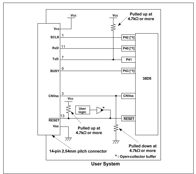
Figure 5.1 Example of an E8a Connection (38D5)
