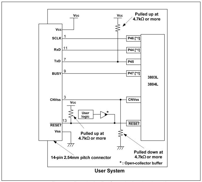
Figure 5.9 Example of an E8a Connection (3803L and 3804L)
