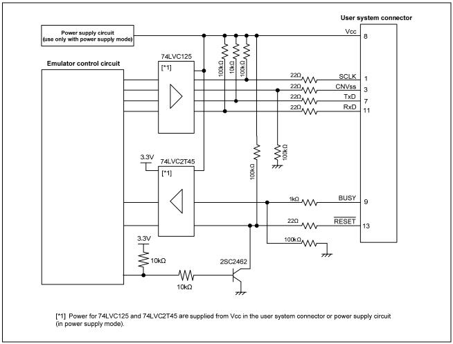
Figure 5.13 Interface Circuit inside the E8a Emulator (For Reference)
