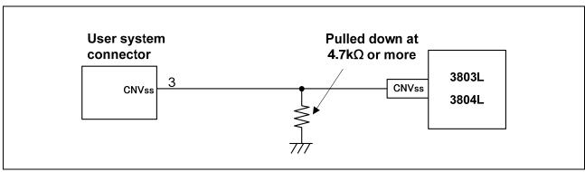
Figure 5.11 E8a Emulator and CNVss Pin Connection
