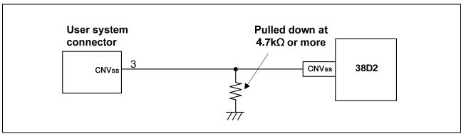
Figure 5.7 E8a Emulator and CNVss Pin Connection
