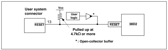
Figure 5.8 Example of a Reset Circuit
