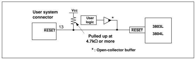
Figure 5.12 Example of a Reset Circuit
