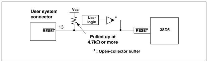
Figure 5.4 Example of a Reset Circuit
