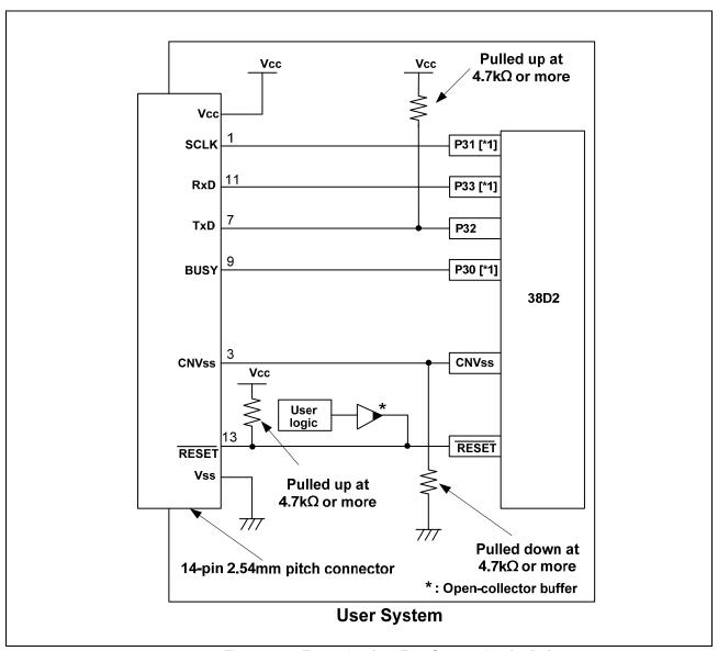
Figure 5.5 Example of an E8a Connection (38D2)
