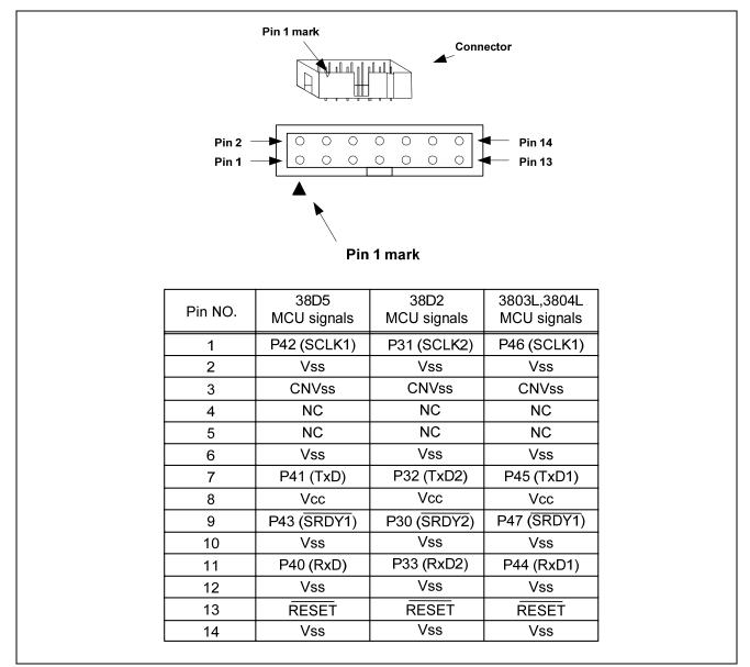
Figure 4.1 E8a Connecting Connector Pin Assignments
