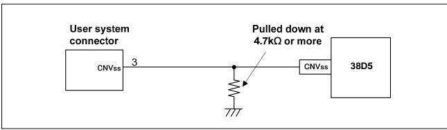
Figure 5.3 E8a Emulator and CNVss Pin Connection
