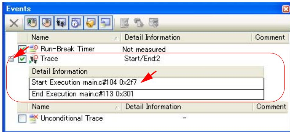
**Remarks 1.** If either one of a trace start event and a trace end event is set as [Valid state](#), the check box of Unconditional Trace event in the [Events panel](#) is automatically cleared, therefore, trace data collection does not automatically start with the start of the program execution (the tracer will not run until the condition of the trace start event that has been set is met).
