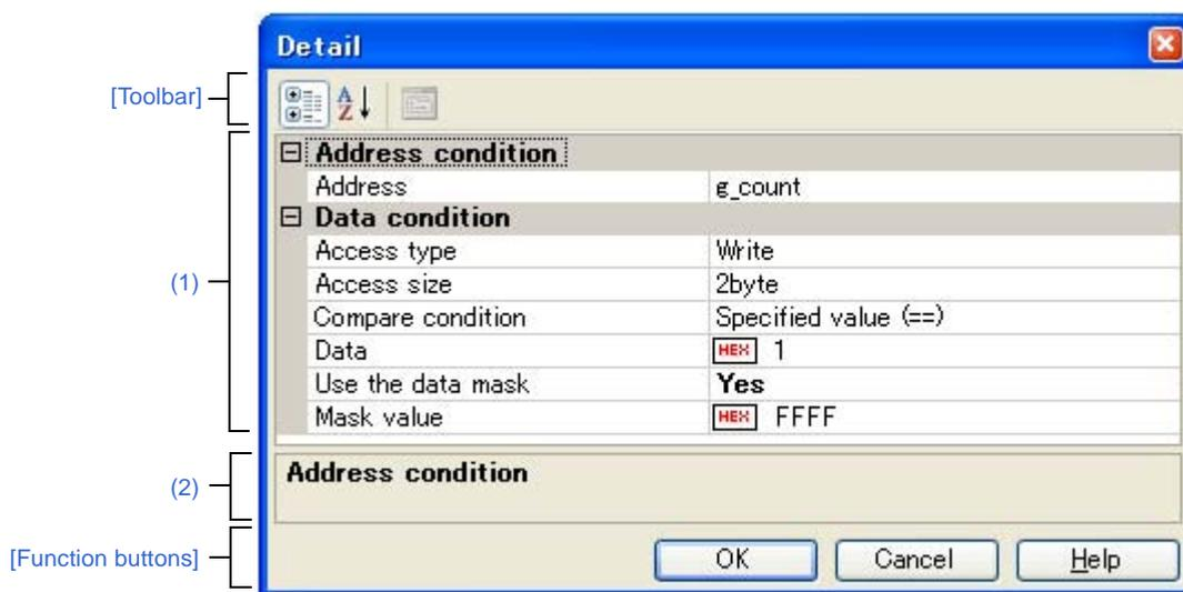
Figure A-61. Detail Dialog Box (for Access Events) [Simulator]
