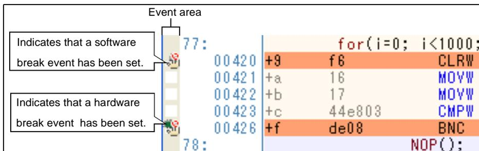
**Figure 2-93. Example of Setting Hardware Break Event (Execution Type) in Events Panel**
