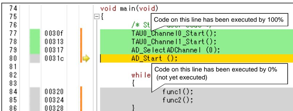
Figure 2-148. View of Code Coverage Measurement Result (Disassemble Panel)
