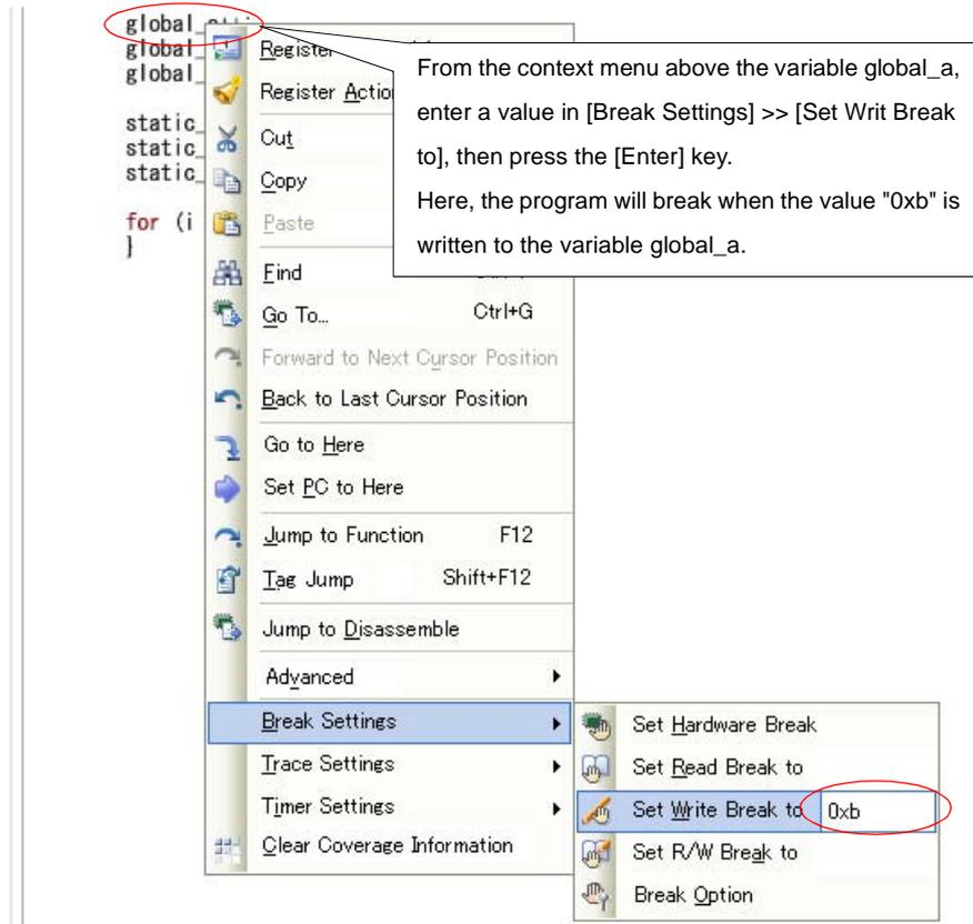
Figure 2-96. Example of Setting Combination Break Event (Access Type) on Variable in Editor Panel [E1][E20]
