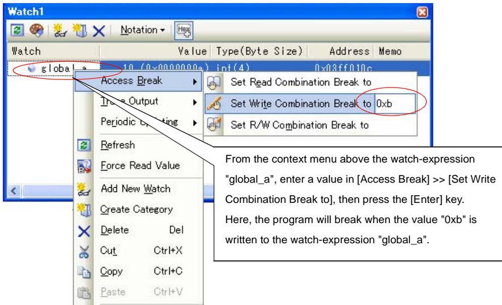
When you have performed the above operation, the set break event (access type) is managed in the [Events panel](#) as a Hardware Break event (access type) or a execution-related event in the detailed information on a Combination Break event (see "2.15 [Manage Events](#)" for details).
