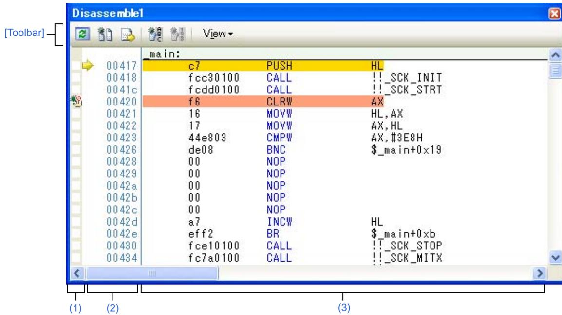
Figure A-25. Disassemble Panel (When Code Coverage Measurement Result Is Displayed)
