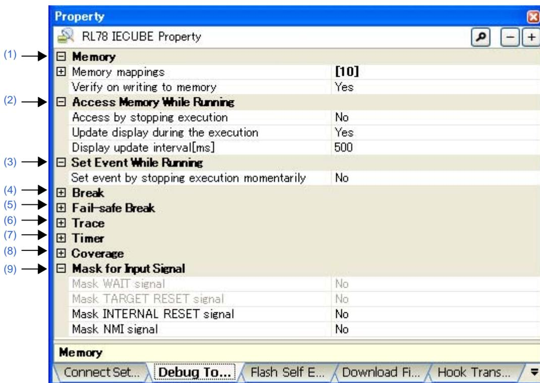
Figure A-9. Property Panel: [Debug Tool Settings] Tab [E1][E20][EZ Emulator]
