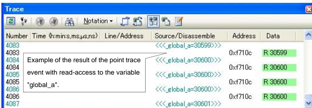
Figure 2-132. Example of Point Trace Event Results View (For 16-bit (2-byte) Variable/SFR) [IECUBE]
