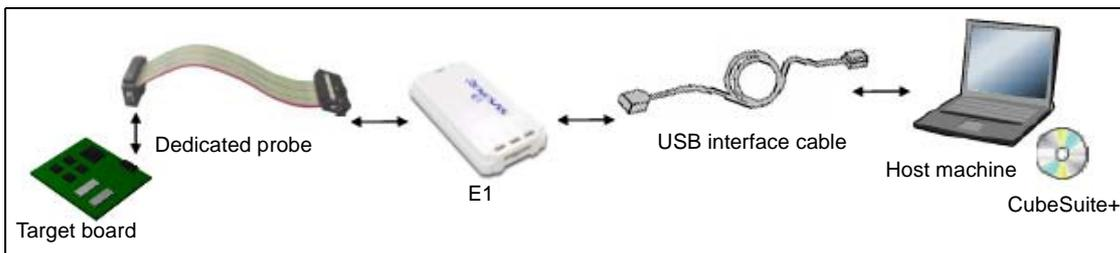
**Caution** Only serial communications are supported as the communication method with the target board (JTAG communications is not available).
