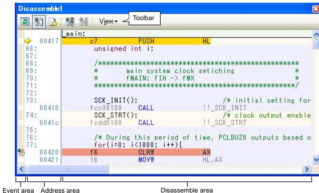
**Remark** You can set the scroll range of the vertical scroll bar on this panel via the [Scroll Range Settings dialog box](#) which is opened by clicking the
