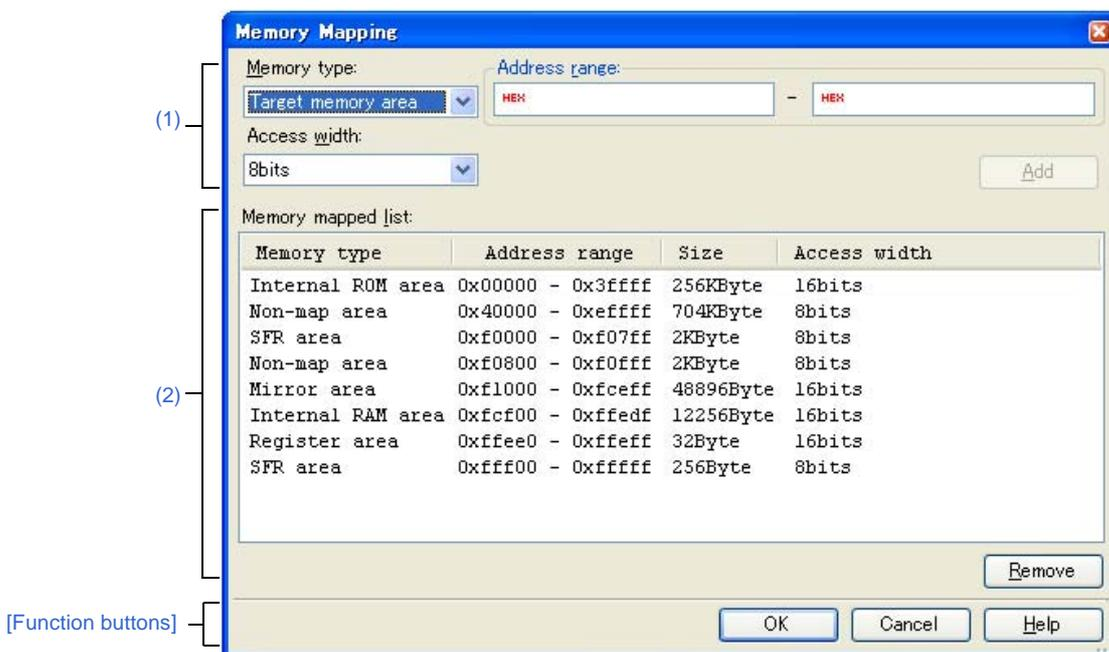
Figure A-37. Memory Mapping Dialog Box [Simulator]
