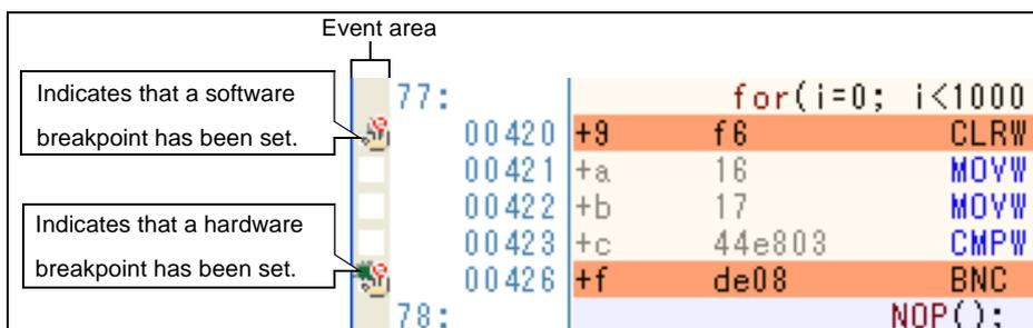
Figure 2-91. Example of Setting Breakpoint in Events Panel
