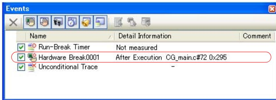
**Figure 2-94. Example of Setting Combination Break Event (Execution Type) in Events Panel [E1][E20]**
