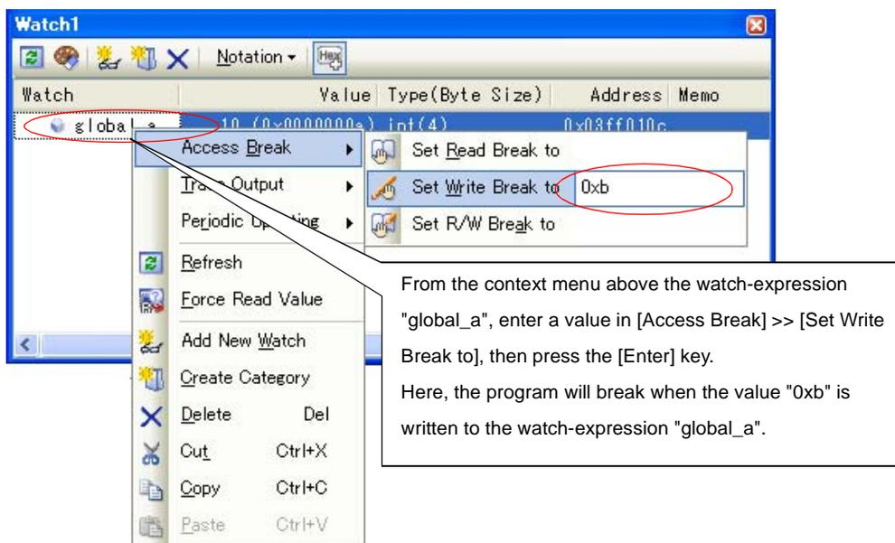
Figure 2-98. Example of Setting Combination Break Event (Access Type) on Watch-Expression [E1][E20]
