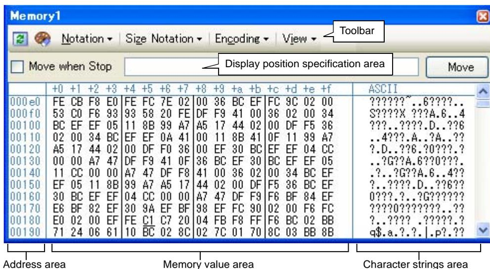
**Remark** You can set the scroll range (as start and end address) of the vertical scroll bar on this panel via the [Scroll Range Settings dialog box](#) which is opened by clicking the button from [View] on the toolbar.
