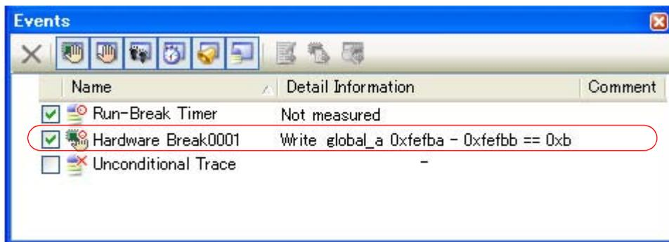
Figure 2-100. Example of Setting Combination Break Event (Access Type) in Events Panel [E1][E20]
