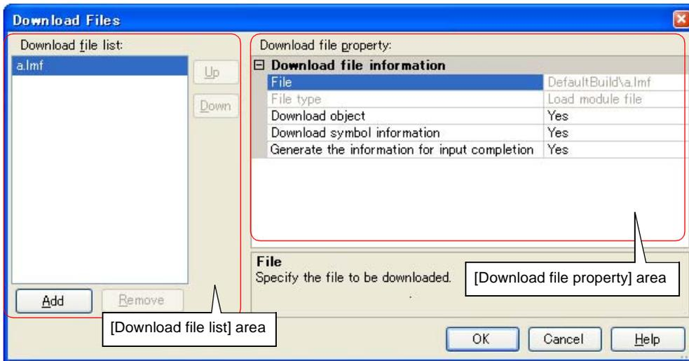
This section describes how to configure on the [Download Files dialog box](#) above when the following cases. For details on the contents and function in each area, see the section for the [Download Files dialog box](#).
