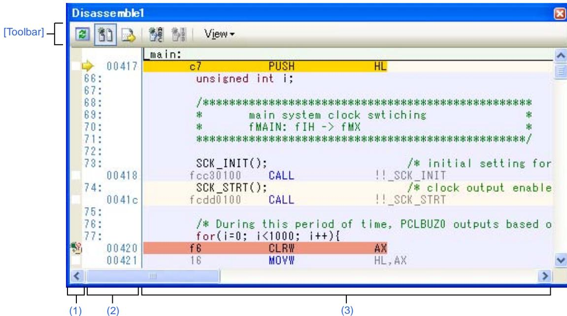
Figure A-24. Disassemble Panel (When Mixed Display Mode Is Not Selected)
