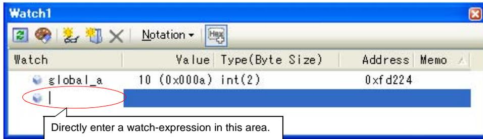
Directly input a watch-expression from the keyboard in the entry box then press the [Enter] key.
