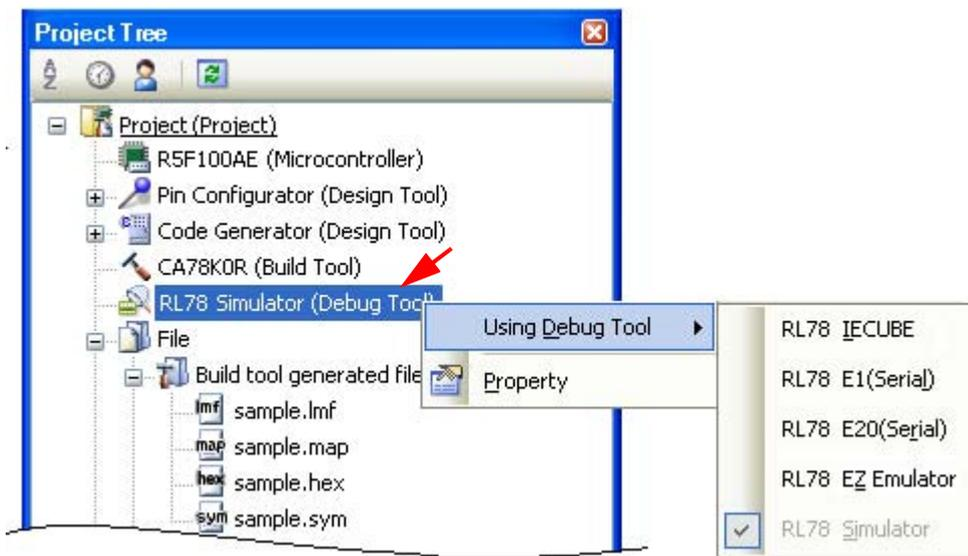
If the [Property panel](#) is already open, click the [RL78 *Debug tool name* (Debug Tool)] node again. The view switches to the Property panel of the selected debug tool.
