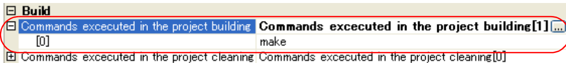
Figure F-16. [Commands executed in the project building] Property (After Setting Commands)
