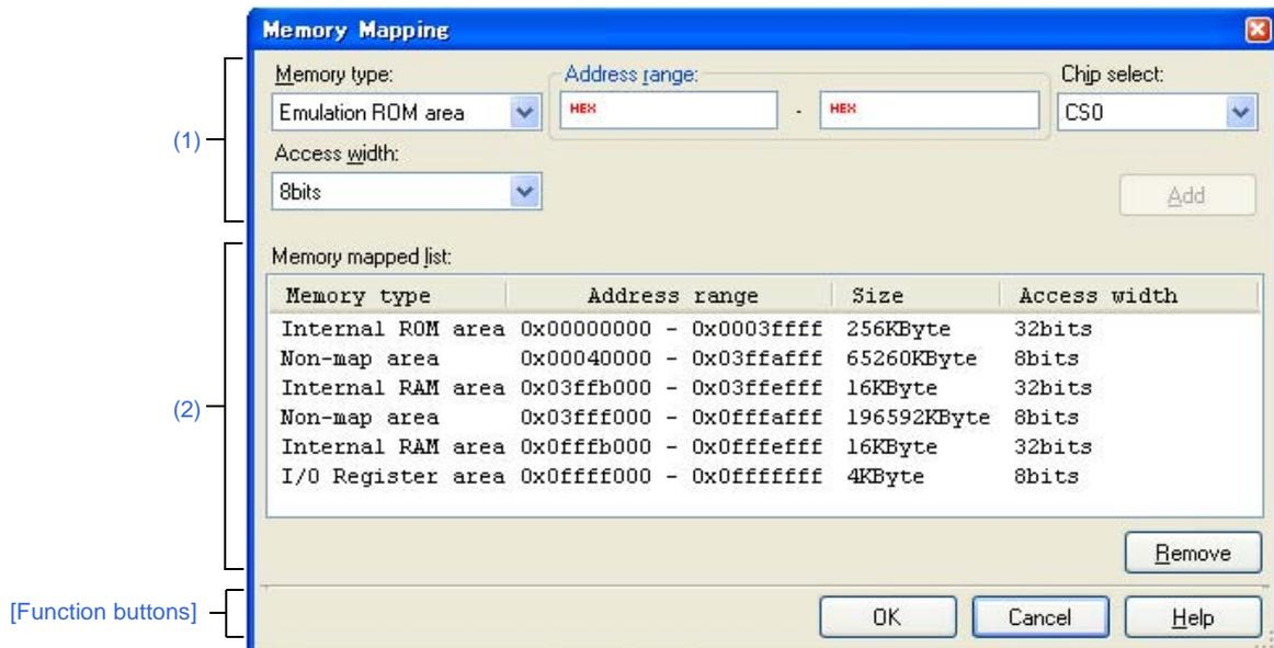
Figure A-52. Memory Mapping Dialog Box [Simulator]
