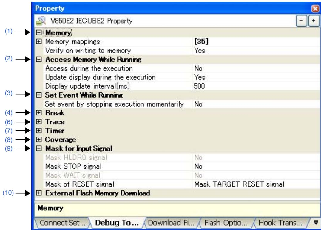
Figure A-16. Property Panel: [Debug Tool Settings] Tab [MINICUBE][E1/E20(JTAG)] ([V850E1][V850ES])
