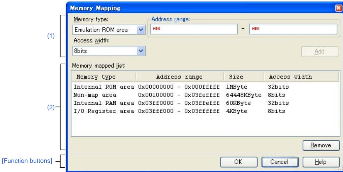
Figure A-51. Memory Mapping Dialog Box [IECUBE[V850E1]]
