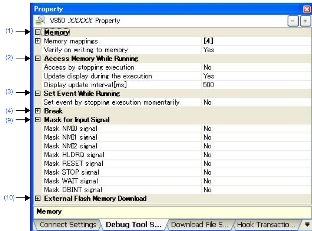
Figure A-17. Property Panel: [Debug Tool Settings] Tab [MINICUBE][E1/E20(LPD)/(JTAG)] ([V850E2])
