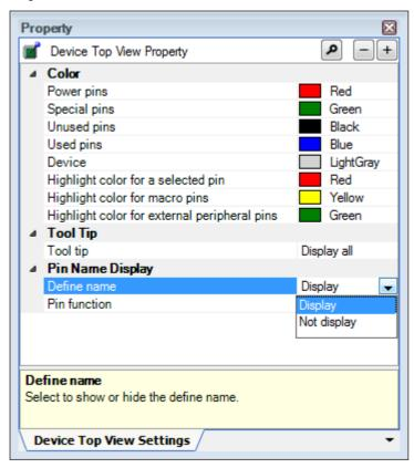
Remark 1. Select one of the following two types for Define name (whether to display the "Define Name" string of the Device Pin List in appended format).
