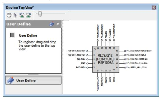
Remark In the Property panel, on the [Pin Configurator Settings] tab, if "BGA" is selected for the Package type, then Device Top View panel cannot be opened.
