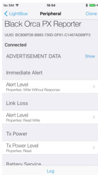
Figure 11: LightBlue application connected to Proximity Reporter application
