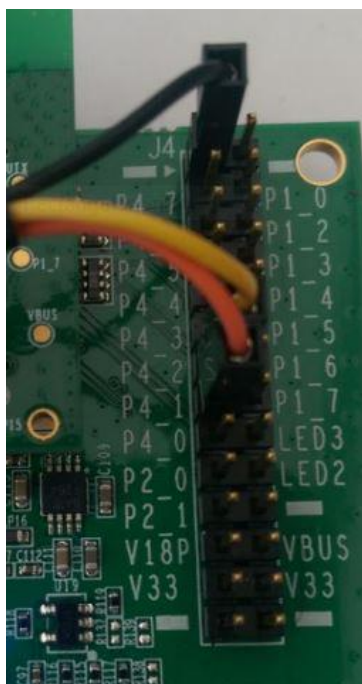
Figure 16: Connecting USB-UART cable to UART2
