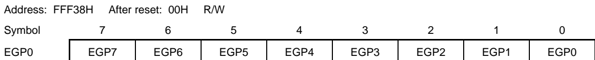
Figure 16-5. Format of External Interrupt Rising Edge Enable Registers (EGP0, EGP1) and External Interrupt Falling Edge Enable Registers (EGN0, EGN1)
