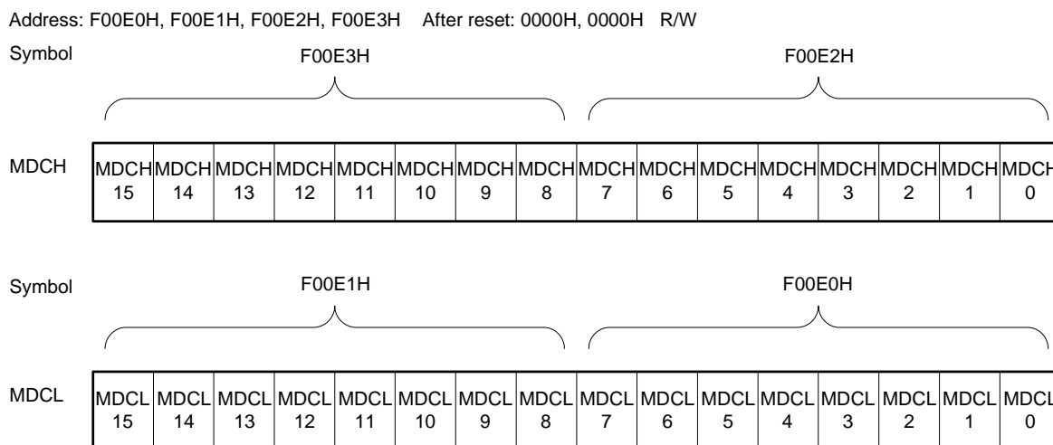
Figure 14-4. Format of Multiplication/Division Data Register C (MDCH, MDCL)
