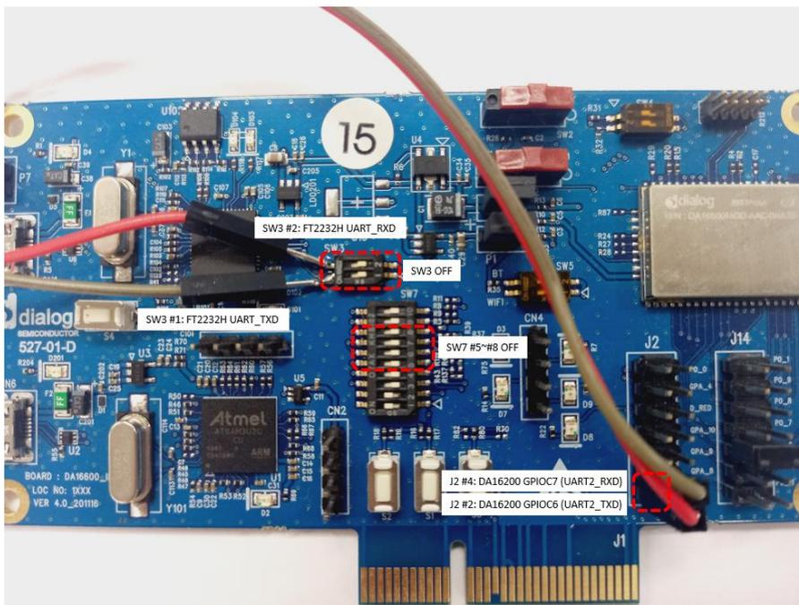
Figure 33: Setting for AT Command over UART (UART2) on EVB 4v0
