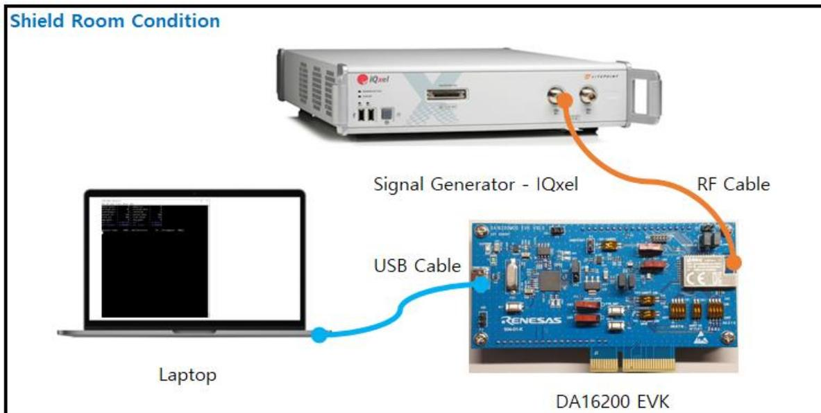
**Figure 28: Setup for RX Test**
