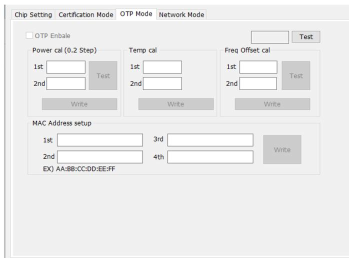
Figure 5: OTP Mode in AT GUI Tool
