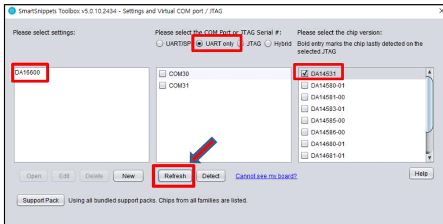
Figure 14: Find Connected COM Port with Refresh
