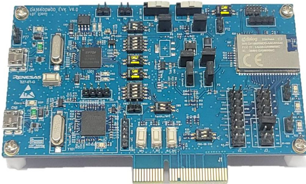
Figure 8: DA16600 EVB Setup for Bluetooth® LE Test
