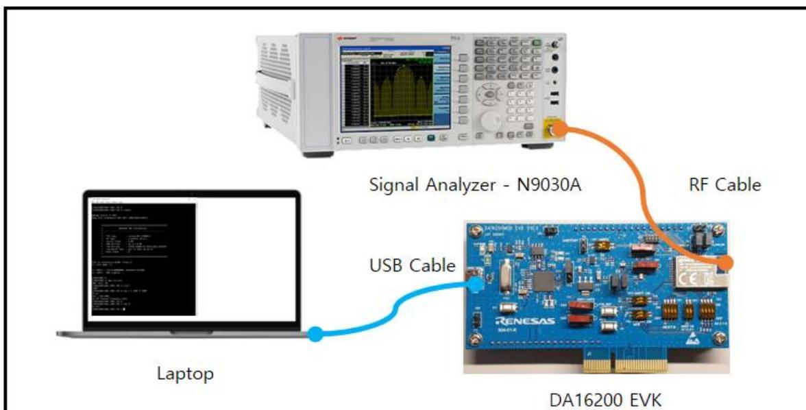
Figure 26: Setup for TX Test
