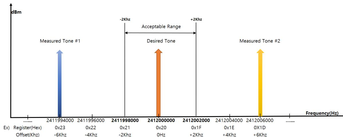
**Figure 2: Offset in Frequency Domain**
