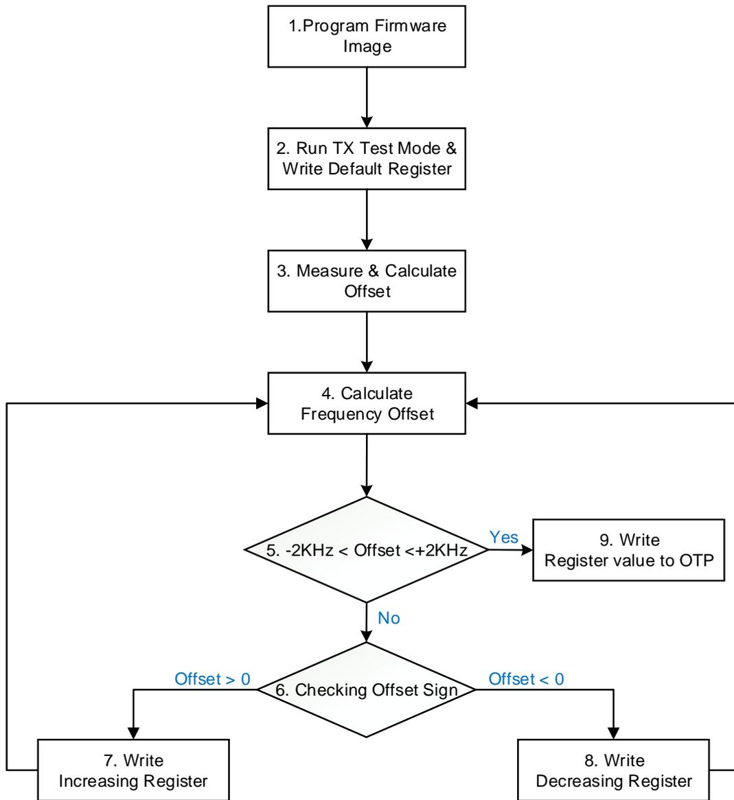
Figure 3: Procedure of XTAL Calibration
