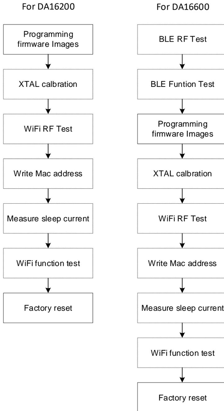
**Figure 1: Flow of Production Test for DA16200/DA16600**
