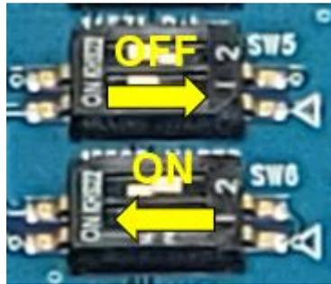
Figure 10: SW5 and SW6 Setup
