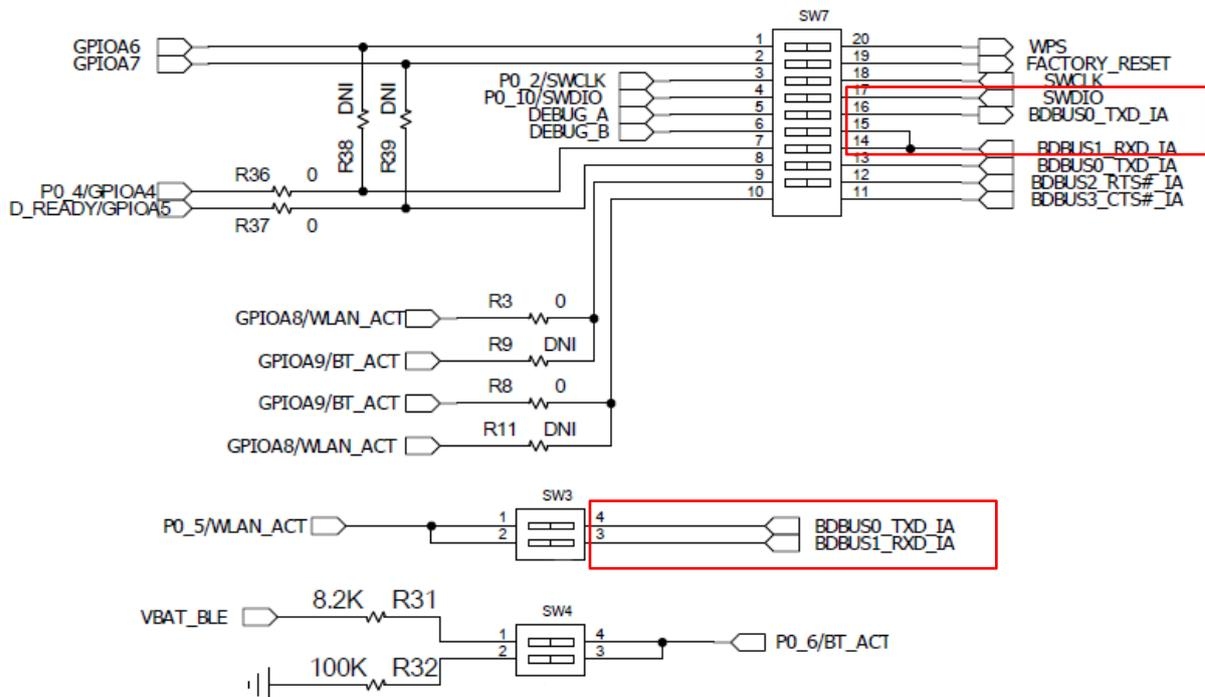
Figure 31: SW3 and SW7 UART1 Connection
