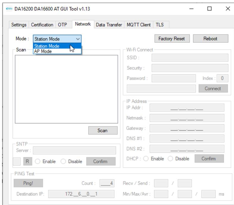
Figure 6: Network Mode in AT GUI Tool
