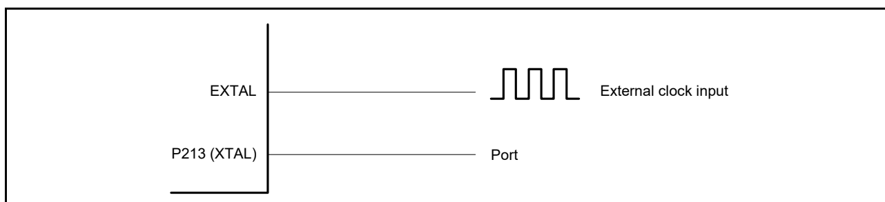
Figure 9.8 Equivalent circuit for external clock
