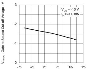
T<sub>ch</sub> - Channel Temperature - °C
